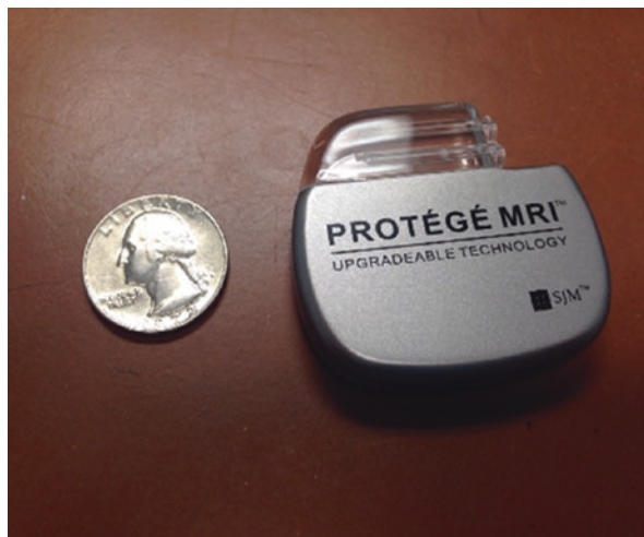
Fig. 11.5 St. Jude Medical Protégé™ rechargeable IPG, conditionally MRI safe for head and extremity MRI scan. (With permission from St. Jude Medical, St. Paul, MN)
