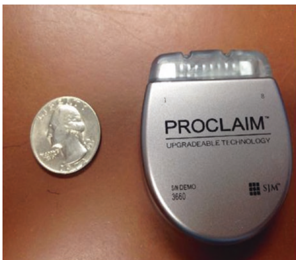
Fig. 11.4 St. Jude Proclaim™ primary cell IPG. (With permission from St. Jude Medical, St. Paul, MN)
