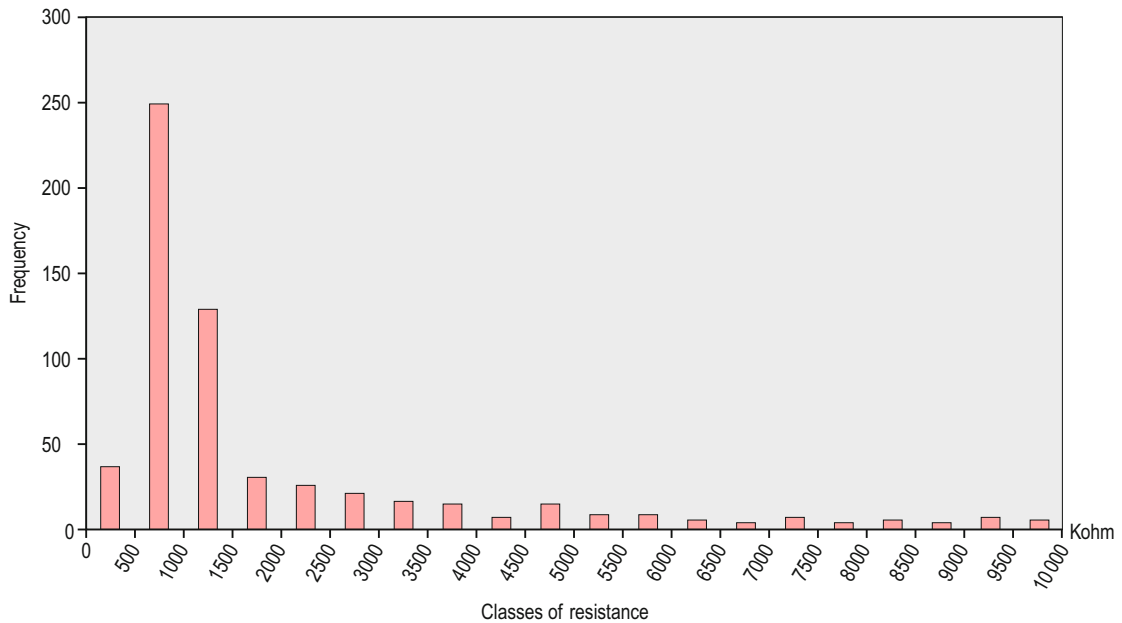
Fig. 6.10 Enlargement of left section of the histogram in Figure 6.7. Only points with resistance lower than 10 000 K \Omega are included.
