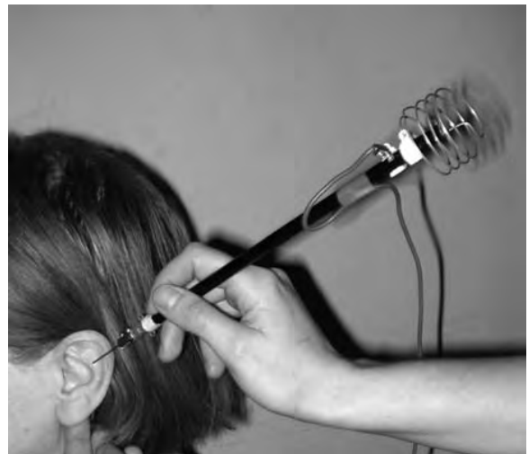
Fig. 6.4 Simple implementation of the hand-held probe, with an external spring to keep constant pressure on skin.
