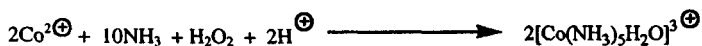
Figure 6.8 Separation of cobalt from nickel solutions using hydrogen peroxide in the presence of ammonia.
