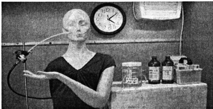
Fig 6.6: COGen 4 on fume cupboard test bench with acid bottles and CO monitor
