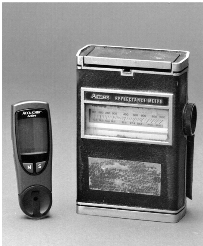
14. Ames Reflectance Meter (1970), the first device for measuring blood glucose outside the laboratory. On the left is one of the many meters available in 2000.
