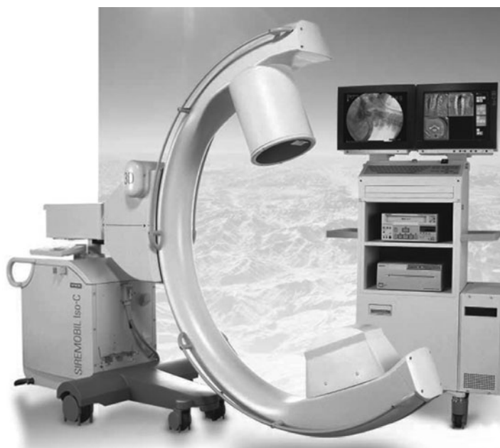
Figure 9.1. X-ray fluoroscopy machine. The C-arm structure of this Siremobil system from Siemens allows the operator to easily obtain an X-ray from any direction by rotating the C-arm around the patient table. The images are captured in the fluoroscope and shown on a video screen in real time. This advanced Iso-C 3D model provides a significant new technical advance: It can actually make a single-slice cross-sectional image similar to the image from a CT scanner. Reprinted with permission of Siemens AG.
