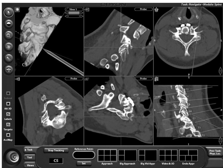
Figure 15.7. Computed-image guidance. This CBYON guidance computer is being used to plot a course for placement of a cervical lateral mass screw. The three-dimensional reconstruction capabilities of the system allow the surgeon to identify and follow a safe course through the bone of the vertebra.
