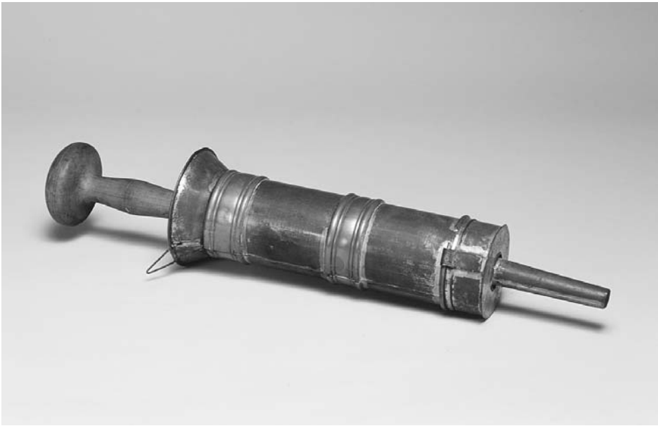
Sausage stuffer. Berks County, Pennsylvania, circa 1860. Wood handle, tin and copper. Ground meat was pressed through the tube into a gut, which was then twisted to make sausages. ROUGHWOOD COLLECTION. PHOTO CHEW & COMPANY.
