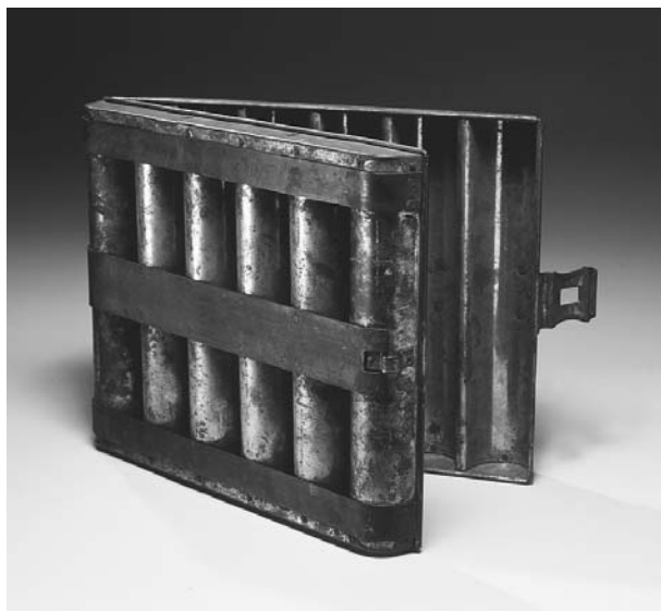
As bread baking became industrialized during the nineteenth century, professional bakers turned to baking aids like this cream loaf pan of tinned sheet iron, which simultaneously makes six large sandwich “batons.” The loaves are perfectly round for slicing. Manufactured about 1890 by Thomas Mills Brothers of Philadelphia. ROUGHWOOD COLLECTION. PHOTO CHEW & COMPANY.
