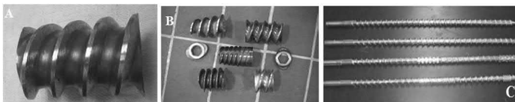
FIGURE 38.3 Screw design. (A) A screw element; (B) typical screw elements; (C) screw is formed by attaching several elements together in various configurations. (From Moscicki [22].)
