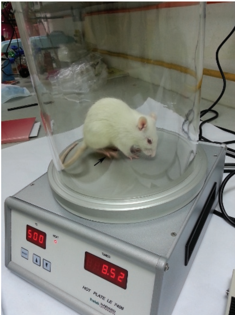
FIGURE 1.5 Hot plate apparatus comprises of an open-ended cylindrical space with a floor of heated plate. Skin of the plantar surface of the foot was stimulated by gently placing the rat on the heated surface. Thermal nociception was evaluated by observing the withdrawal reflex latency (WRL) of the operated limb in response to heat stimulation (as indicated by an arrow) by a built-in timer activated by an external foot switch. (Reprinted from Wong, Kah-Hui et al . Restoration of sensory dysfunction following peripheral nerve injury by the polysaccharide from culinary and medicinal mushroom, Hericium erinaceus (Bull.: Fr.) Pers. through its neuroregenerative action. Food Sci. Technol (Campinas) , Campinas , v. 35, n. 4, p. 712-721, Dec. 2015 . Available from http://www.scielo.br/scielo.php?script=sci_arttext&pid=S0101-20612015000400712&lng=en&nrm=iso https://creativecommons.org/licenses/by/4.0/deed.en )
