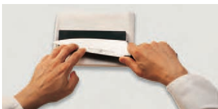
(d) Draw the knife across the stone all the way to the heel of the blade.
