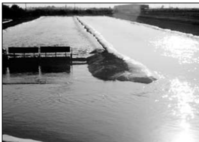
B.12. A paddlewheel circulates water around a pond.
