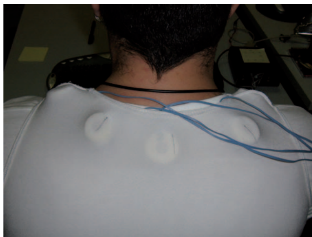
FIGURE 17.4 The vibrotactile BCI: Feedback was provided via vibrotactile transducers mounted around the neck between two T-Shirts. A contactor in the centre of a magnetic coil through which current was flowing moved against the skin and back at a frequency of 200Hz. Imagery of right hand movement activated the contactors on the right hand side of the neck and imagery of left hand movement those of the left hand side. Source: The photograph is with kind permission from Dr. Febo Cincotti, Laboratory of Neuroelectrical Imaging and Brain Computer Interface, Fondazione Santa Lucia IRCCS, Rome, Italy.
