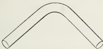
FIG. 19. Tube properly Bent.
