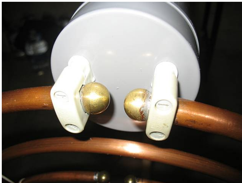
Connection of antennas to the Tesla coils
