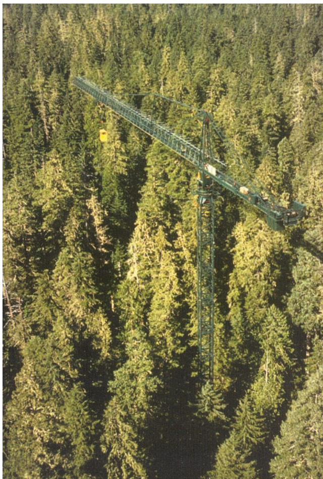
FIG. 16.4 Canopy cranes are a new tool for experimental access to forest canopies. For example, the gondola of the Wind River Canopy Crane (75-m tall tower, 84-m long jib) can access 700,000 m 3 of 60-m tall canopy, as well as the canopy-atmosphere interface, over a 2.3-ha area in a 500-year-old Pseudotsuga/Tsuga forest in southwestern Washington, United States. Photo by J. F. Franklin, from D. Shaw (2004). Please see extended permission list pg 573.
