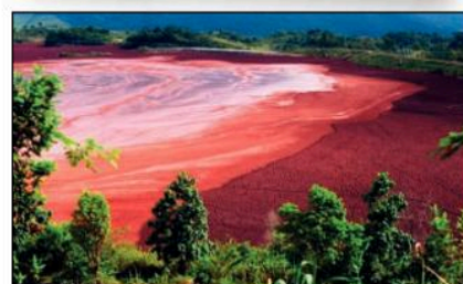
Figure 2.2.4 This waste pond is a mixture of water and chemical waste from the extraction of aluminium.
