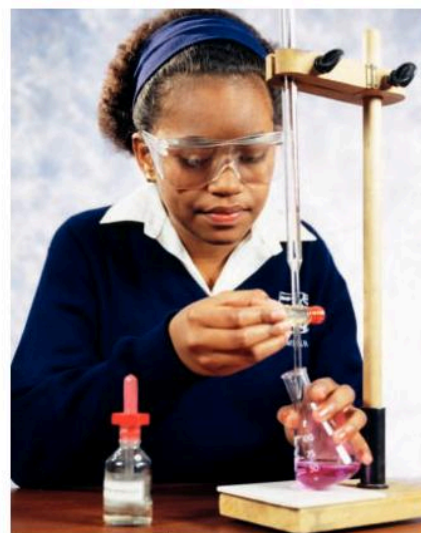
Figure 7.8.2 The results from a titration can be used to calculate the concentration of an acid or alkali.
