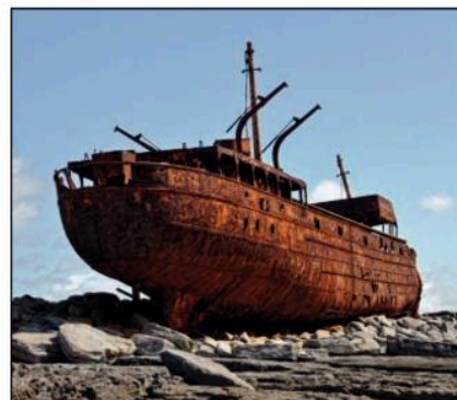
Figure 8.3.1 Ships' hulls rust easily in the presence of water and air.
