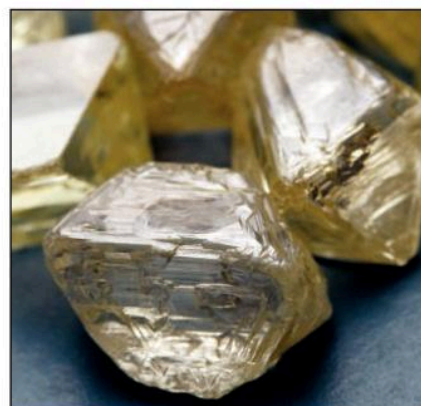
Figure 5.5.3 Diamonds are hard and long-lasting because of the network of strong covalent bonds in the structure.
