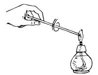
and repeat the process on the other end. CAUTION: If you keep the glass in the flame for too long, it will melt, the hole will close, and you will have a closed tube instead of an open one.
