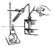
*Results:* There was no flame inside the test tube containing wood. Since you did not apply flame directly to the wood, it didn't reach its kindling point. Nevertheless, you could see that it was being burned up. The heat was great enough to force certain chemicals out of the wood. These collected in the form of the yellowish liquid in the second test tube. When you brought a match near the nozzle, the gas escaping from the yellow liquid ignited.
