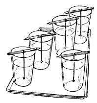
in, move them to a slightly cooler place. Move the whole tray at once and do it gently, so that the contents of each glass remain undisturbed. After an hour, move them to a still cooler place, perhaps the refrigerator. Lowering the temperature gradually and moving the tray without disturbing the contents of the glasses is extremely important for the success of this experiment. Once the solutions have cooled to about  $40^{\circ}$  F., let them stand for several days.
