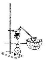
Allow most of the liquid to boil away. Note the color of the liquid collected in the jar.
