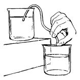
Submerge the tube in the upper container so that it is completely filled with liquid. Keep one end of the tube submerged and, holding the other end closed, lower it into the empty container. When you open the tube, the liquid will flow.
