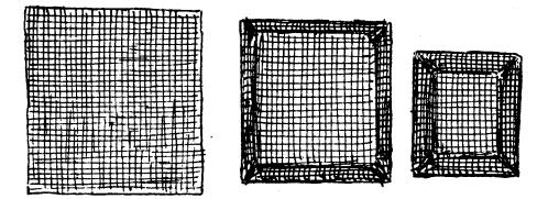
Now you have a wire gauze pad which can withstand the heat of your alcohol burner, and which will not endanger your fingers while you are using it. To use it, you place it over the ring support and rest on it the container you wish to heat. You will probably want several wire gauze pads.
