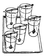
the same shape and had the same general appearance regardless of size. Crystals tied on the string were *seed* crystals. They provided surfaces for the others to grow around. When the solutions cooled, some of the solute separated out in crystalline patterns, characteristic of the particular solute.
