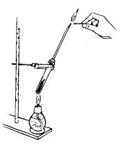
**Results:** When you heated the coal, it gave off the gases, mainly methane  $(CH_4)$  and ethane  $(C_2H_6)$ , that were trapped in it as it was formed in the earth. This gaseous mixture burned with a characteristic blue flame. The material which remained in the test tube is a form of carbon called *coke*. If there was any sticky brownish substance there, too, it was a combination of *coal tar* products, which are the residue of coal burned in this way.
