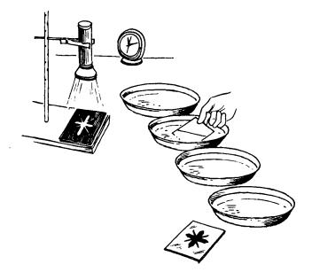
Repeat this procedure with each of the photographic plates. You may find that varying time intervals and different thicknesses of the gelatin coating produce more or less successful results. You will want to experiment a bit until you find the best time exposure for the plates you have made.
