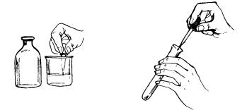
How to Measure a Liquid. If you look through the side of a measuring glass filled with a liquid, you will see that the surface of the liquid has a double curve. This curve is called the *meniscus*. In measuring, be sure to use the lowest part of the lower curve. Most liquids have a *concave* meniscus (one that curves downward) but very dense liquids like mercury have a *convex* meniscus (one that curves upward). In that case, use the uppermost part of the upper curve for measuring.
