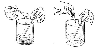
stirring the solution all the time. If the solution becomes dark blue, you will have to start all over again. When the ammonium hydroxide ceases to make the solution turn any lighter, pour the liquid through a funnel lined with filter paper into the third jar. Now put the filter paper and everything caught in it into the fourth jar. Add just enough concentrated ammonium hydroxide to dissolve the filter paper. Pour 11 tablespoonfuls of dilute sulfuric acid into the
