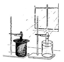
with a diameter a little larger than the diameter of a test tube. Put this piece of paper over the surface of the hydrogen peroxide. Now fill the covered test tube with hydrogen peroxide and put it, upside down, through the hole in the paper-covered jar, as you did before.
