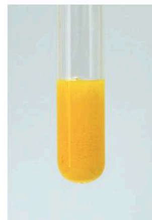
► Figure 22.1.2 A bright yellow precipitate forms when potassium iodide solution is added to a solution containing \text{Pb}^{2+} ions
