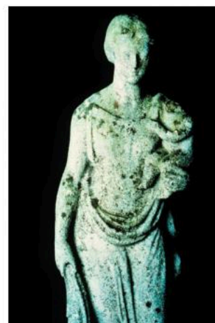
▲ Figure 20.5.2 A limestone statue corroded by acid rain
