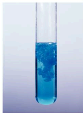
▲ Figure 22.1.1 A blue precipitate forms when sodium hydroxide solution is added to a solution containing Cu 2+ ions
