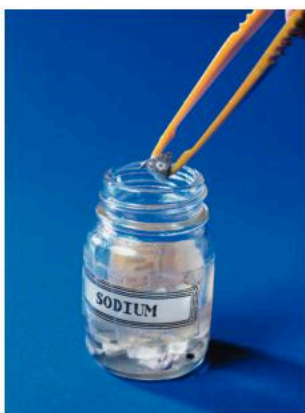
▲ Figure 17.2.1 Sodium has to be stored under paraffin to prevent it from reacting with oxygen in the air
