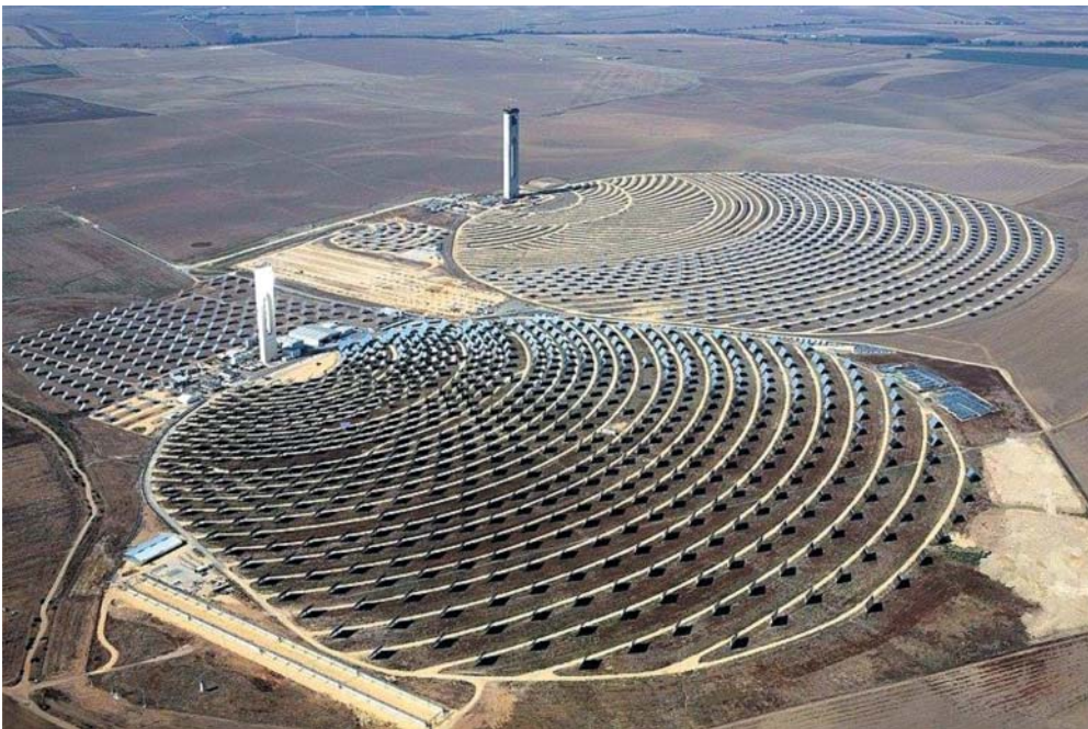
Figure 13.12 The PS10 (left) and PS20 (right) concentrated solar power stations located in Andalusia, Spain. Source: Koza 1983, Wikimedia Commons.
