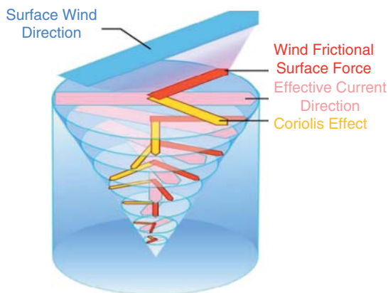
Figure 8.6 An Ekman spiral caused by the effects of surface winds interacting with the Coriolis force to create a spiral upwelling event. Source: Adapted from Timer, Wikimedia Commons.
