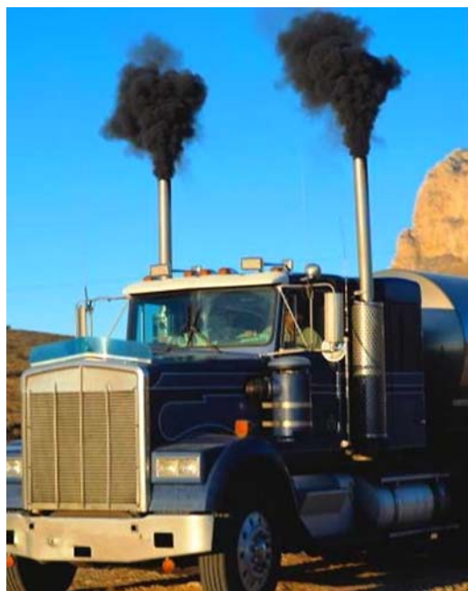
Figure 10.22 The emission of a large amount of diesel soot from a heavy duty diesel truck during engine start-up. Source: USEPA, Wikimedia Commons.
