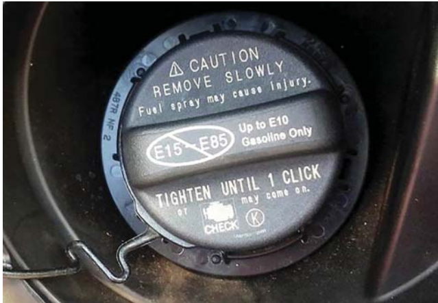
Figure 10.12 The gas cap of a 2012 Toyota Camry showing a warning against using gasoline–ethanol blends higher than E10 in the vehicle. Source: Mario Roberto Durán Ortiz, Wikimedia Commons.
