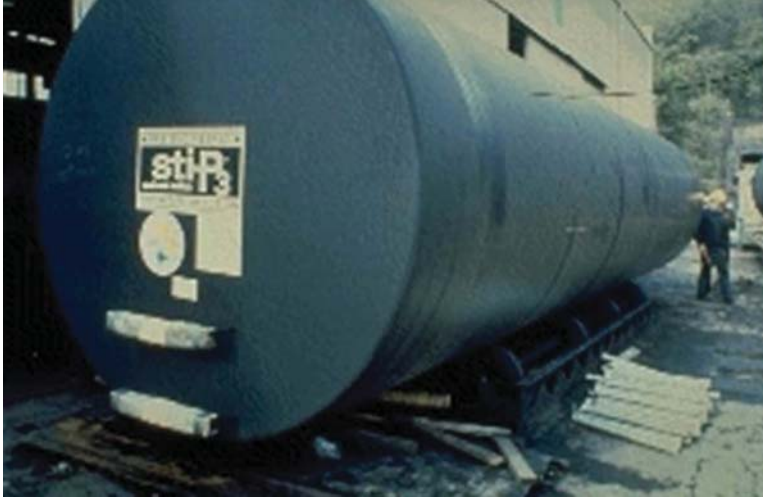
Figure 10.16 A polymer-coated steel petroleum underground storage tank (UST) showing white metal bars attached to the steel, which act as sacrificial anodes for cathodic protection of the tank. Source: U.S. Environmental Protection Agency, Wikimedia Commons.
