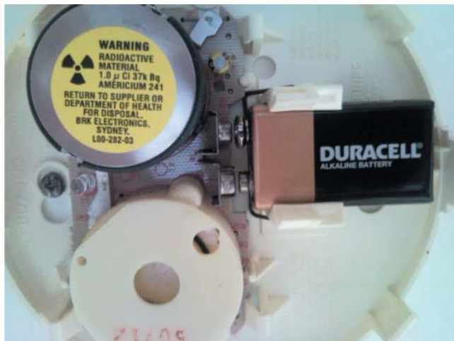
Figure 12.25 The inside of a typical household smoke detector showing the labeled ^{241}\text{Am} \alpha source used to produce ionized smoke particles. Source: MD111, Wikimedia Commons.
