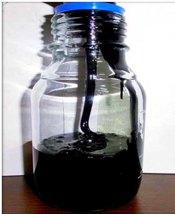
Figure 10.21 Number 6 heavy distillate fuel oil known as Bunker C. Source: Glasbruch 2007, Wikimedia Commons.
