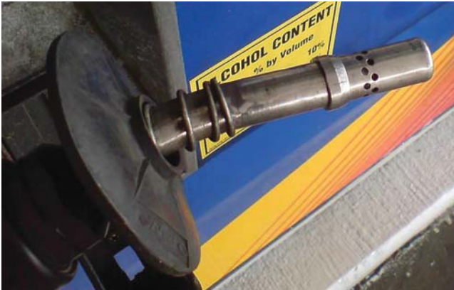
Figure 10.24 A gasoline dispensing nozzle with a rubber gasket used to capture gasoline vapors and return them to the underground storage tank. Source: Mroach, Wikimedia Commons.
