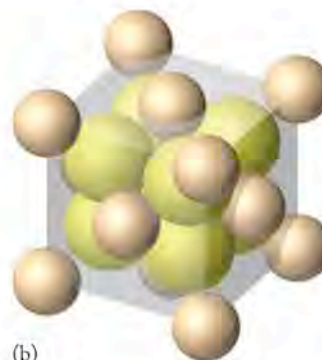
FIGURE 11.25 (a) The cubic structure of the ions in the mineral fluorite ( CaF_2 ) can produce beautiful, nearly transparent cubic crystals. (b) The crystal structure of CaF_2 is based on an fcc array of Ca^{2+} ions, with F^- ions occupying all 8 tetrahedral holes. However, F^- ions are bigger than Ca^{2+} ions, so they do not fit in the normal tetrahedral holes of a cubic closest-packed array of Ca^{2+} ions. Instead, the Ca^{2+} ions spread out to accommodate the larger F^- ions while maintaining an fcc structure.
