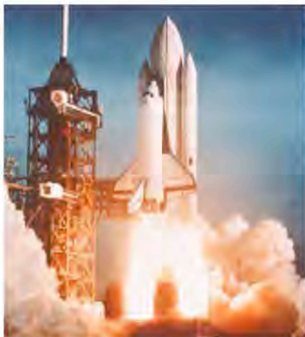
At full throttle, each of the three main engines of a U.S. space shuttle produces about 12 million horsepower ( 9 \times 10^6 \text{ kJ/s} ) as it burns liquid hydrogen at a rate of about 1,100 L (38,000 mol) per second.
