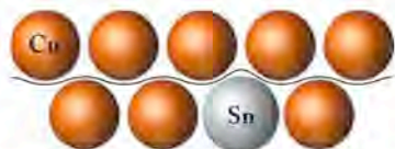
FIGURE 11.13 The larger Sn atoms in bronze perturb the crystal structure of Cu atoms, producing atomic-scale bumps in the slip plane (wavy line) between layers of Cu atoms. These bumps make it more difficult for Cu atoms to slide by each other when an external force is applied, and that makes bronze tools and weapons harder and stronger than those made of pure copper.
