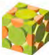
FIGURE 11.23 (a) Sodium chloride forms cubic crystals that sometimes reach impressive size. (b) The NaCl crystal structure is based on an fcc unit cell that the Cl^- ions adopt, with Na^+ ions occupying the octahedral holes. (c) Ions at the corners and faces and along the edges are shared with other unit cells. As shown in this cutaway view, only fractional portions of ions at these positions are assigned to a single unit cell.
