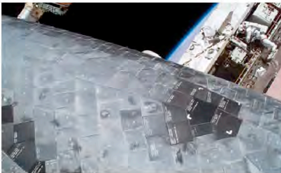
FIGURE 11.31 About 25,000 heat-resistant tiles cover much of the surface of each U.S. space shuttle, protecting it from re-entry temperatures of over 1100°C. Most tiles are made of high-purity, amorphous SiO 2 fibers. Ninety percent of each tile is open space between the fibers, which means that the tiles are both lightweight and highly resistant to high temperatures.
