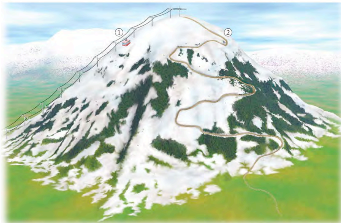
FIGURE 5.2 Work is done as skiers ascend to the top of a mountain. The amount of work differs, depending on whether a skier (1) rides a gondola on a direct route to the top or (2) hikes to the top along a winding path, because the paths taken are of different lengths and work depends on the distance through which a force acts in moving a mass.
