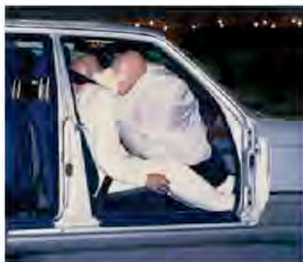
An automobile air bag inflates when solid \text{NaN}_3 rapidly decomposes, producing \text{N}_2 gas.
