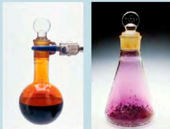
Liquid bromine and solid iodine both have high vapor pressures at typical room temperature.
