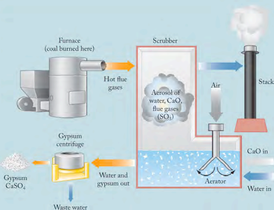
FIGURE 4.21 A scrubber capitalizes on the acid–base chemistry of aqueous solutions of calcium oxide and the oxides of sulfur in order to trap exhaust gases that would otherwise produce strong acid rain if released into the atmosphere.
