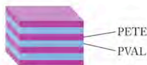
FIGURE 12.17 Layers of the polymers PVAL and PETE are used to make soda bottles.
