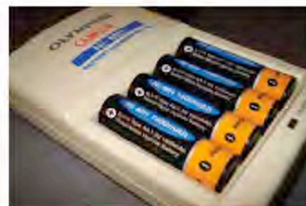
The electrical energy rating of these rechargeable AA batteries is 1.6A · hr at 1.2 V.
