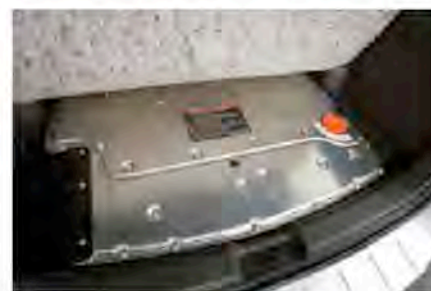
The 2008 Ford Escape is powered by a 133 horsepower gasoline engine and a 94 horsepower (70 kW) electric motor. As in most of the first-generation hybrid vehicles, power for the Escape's electric motor comes from a pack of nickel–metal hydride (NiMH) batteries under the floor.
