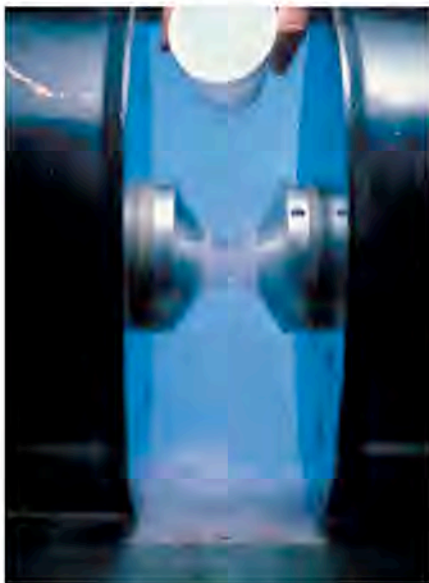
FIGURE 9.29 Molecular orbital theory explains the behavior of liquid oxygen in a magnetic field. The unpaired electrons in the \pi^* orbitals make O_2 paramagnetic, which means it is attracted to a magnetic field, as shown in this picture of liquid oxygen being poured between the poles of a large magnet. Substances composed of diamagnetic molecules in which all electrons are paired do not exhibit this behavior.
