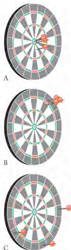
FIGURE 1.17 Accuracy refers to the proximity of a result to the true value. On a target the closer to the bull's-eye the dart lands, the more accurate the throw. Precision refers to the proximity of several results to one another. On the target, proximity is represented by three darts very close to each other. Throws at target A are both accurate and precise; at target B, precise but not accurate; at target C, neither precise nor accurate.
