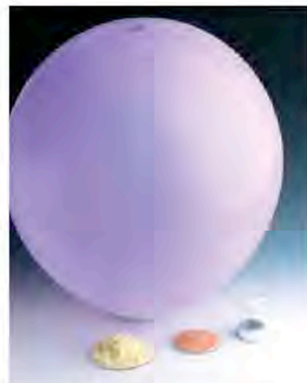
FIGURE 3.3 The quantities shown are equivalent to 1 mole of each material: 4.003 g of helium, 32.07 g of sulfur, 63.55 g of copper, and 200.59 g of mercury.
