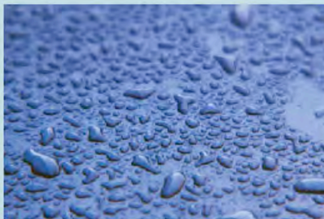
Rain beads on metal treated with a silicone polymer.
