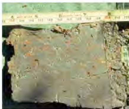
FIGURE 4.17 Wetland soils: (a) the soil in this wetland has a blue-gray color because of the presence of iron(II) compounds. (b) Orange mottling indicates the presence of Fe(III) oxides formed as a result of O_2 permeation through channels made by plant roots.
