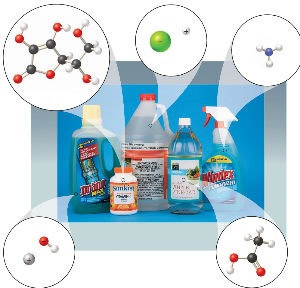
Figure 4.5 Some common acids and bases. From left to right: Sodium hydroxide (NaOH), ascorbic acid ( C_6H_8O_6 or, with its ionizable hydrogens written first, H_2C_6H_6O_6 ), hydrochloric acid (HCl), acetic acid ( HC_2H_3O_2 ), and ammonia ( NH_3 ). HCl and NaOH are both strong electrolytes and exist in solution entirely as ions. Water molecules are not shown.
