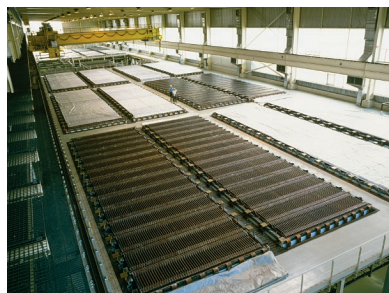
Figure 24.7 Copper cathodes used in the electrorefining process.
