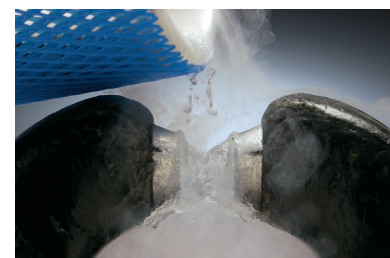
Liquid oxygen is attracted to the poles of a magnet because O 2 is paramagnetic.
