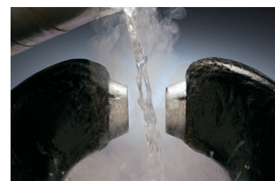
Liquid nitrogen is not attracted to the poles of a magnet because N 2 is diamagnetic.
