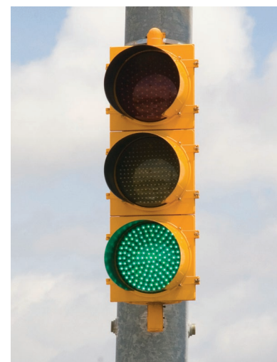
Figure 12.17 LED arrays in traffic signals. Many communities have replaced the red and green signals with LED arrays that are much more energy efficient than the incandescent bulbs used previously. The yellow lights are being replaced more slowly, however, because LED arrays are expensive and the short duration of yellow lights would not necessarily allow an overall cost saving when the energy efficiency is factored in.
