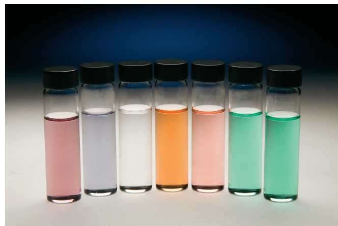
Figure 22.16 Colors of some of the first-row transition metal ions in solution. From left to right: \text{Ti}^{3+} , \text{Cr}^{3+} , \text{Mn}^{2+} , \text{Fe}^{3+} , \text{Co}^{2+} , \text{Ni}^{2+} , \text{Cu}^{2+} . The \text{Sc}^{3+} and \text{V}^{5+} ions are colorless.
