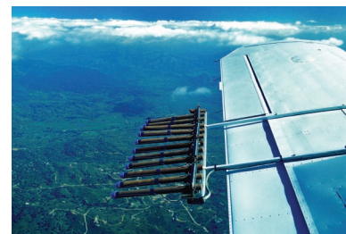
Figure 25.20 Cloud seeding using AgI particles.
