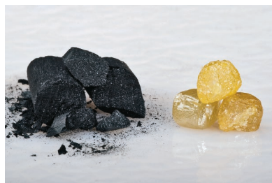
Figure 25.5 A synthetic diamond and the starting material—graphite.
