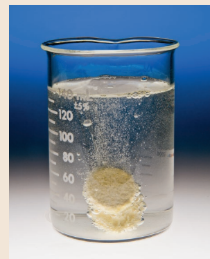
The reaction of sodium bicarbonate and citric acid produces Alka-Seltzer's effervescence.
