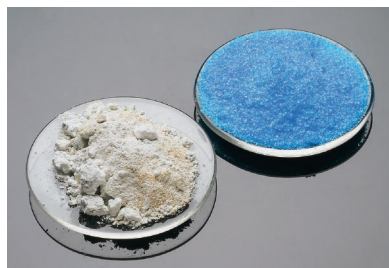
Figure 2.15 \text{CuSO}_4 is white. The pentahydrate, \text{CuSO}_4 \cdot 5\text{H}_2\text{O} , is blue.
