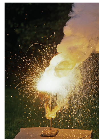
Figure 24.19 The temperature of a thermite reaction can reach 3000^\circ\text{C} .
