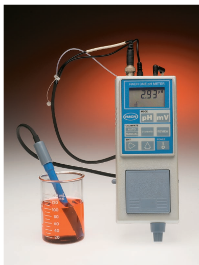
Figure 16.1 A pH meter is commonly used in the laboratory to determine the pH of a solution. Although many pH meters have a range of 1 to 14, pH values can actually be less than 1 and greater than 14.
