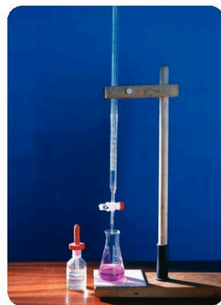
▲ A titration: sodium hydroxide solution was added to hydrochloric acid, from the burette. Neutralisation is complete: the phenolphthalein has turned pink.
