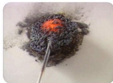
▲ Iron and sulfur reacting: the total mass is the same before and after.
