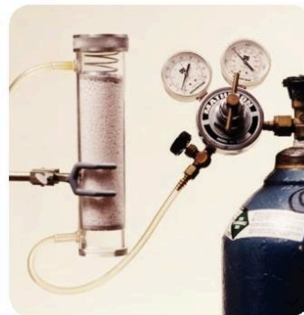
▲ Calcium chloride absorbs water, so it is used to dry gases. The glass cylinder above is packed with calcium chloride, and the gas is piped up through it.
