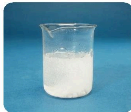
▲ Calcium carbonate reacting with dilute hydrochloric acid. What is that gas?
