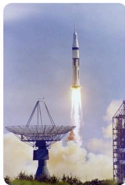
▲ The reaction between hydrogen and oxygen gives out so much energy that it is used to power rockets. The reactants are carried as liquids in the fuel tanks.
