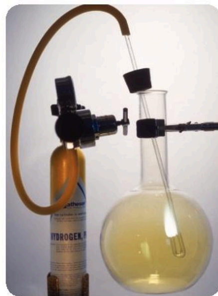
▲ Hydrogen burning in chlorine in the lab. Bonds break and new bonds form, giving hydrogen chloride.
