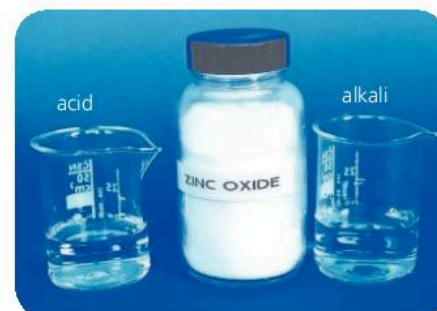
▲ Zinc oxide: an amphoteric oxide. It will react with both acid and alkali.
