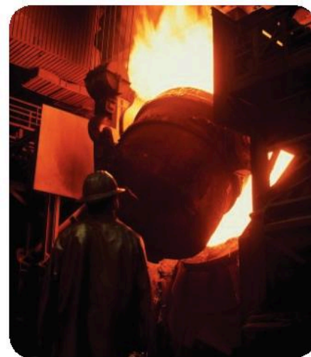
▲ Magnesium oxide is used to line furnaces in steel works, because of its high melting point, 2852°C. (By contrast, iron melts at 1538°C.)
