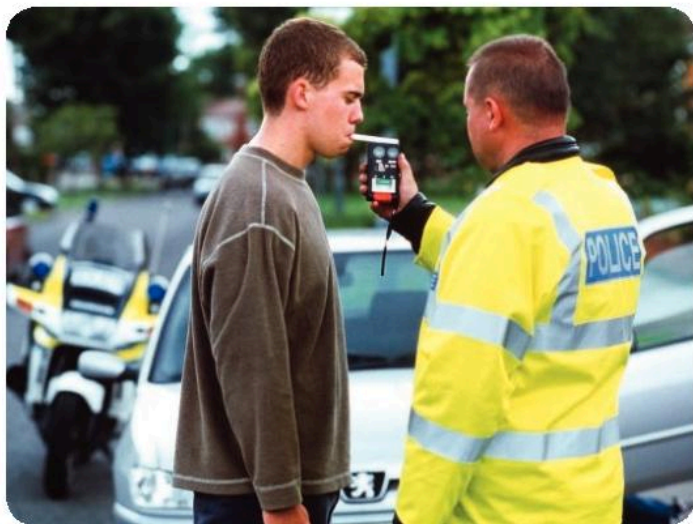
▲ Has he been drinking? Yes or no? Alcohol on the breath will turn orange potassium dichromate(VI) green.
