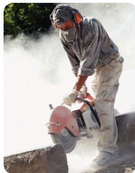
▲ Diamond: so hard that it is used to edge wheels for cutting stone.
