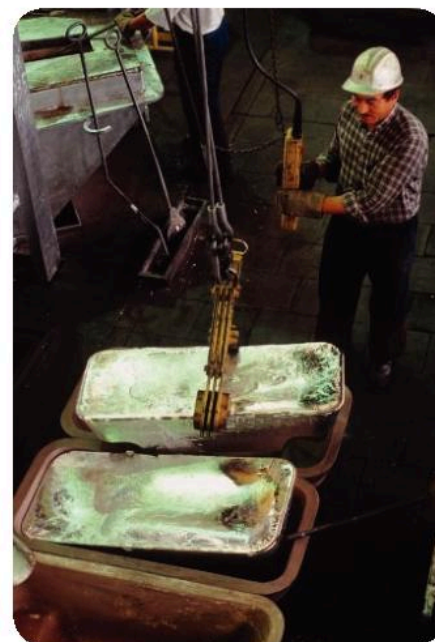
▲ Molten aluminium from the tank was run into these moulds, to make blocks.
