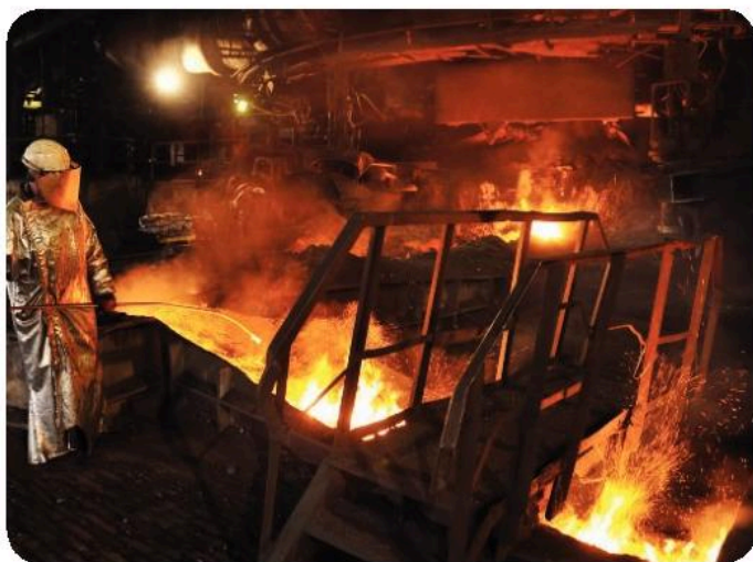
▲ Iron occurs naturally in the earth as iron(III) oxide, \text{Fe}_2\text{O}_3 . This is reduced to iron in the blast furnace. Here, molten iron runs out from the bottom of the furnace.
