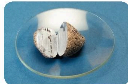
▲ A piece of sodium, cut with a knife.
