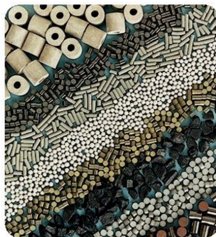
▲ Many different substances can act as catalysts. They are usually made into shapes that offer a very large surface area.
