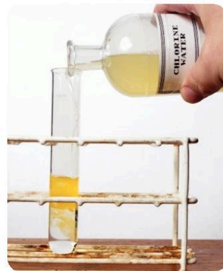
▲ Chlorine displacing bromine from aqueous potassium bromide.
