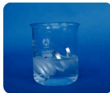
▲ Magnesium displacing hydrogen from hydrochloric acid.
