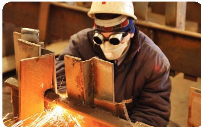
▲ Easy: slicing through steel with an oxy-acetylene flame.
