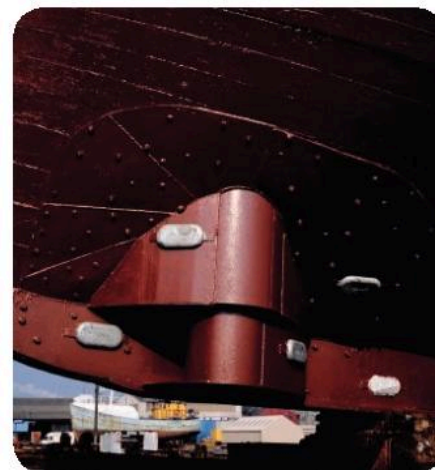
▲ Here blocks of magnesium have been welded to a ship's hull, to prevent the steel (an alloy of iron) from corroding.
