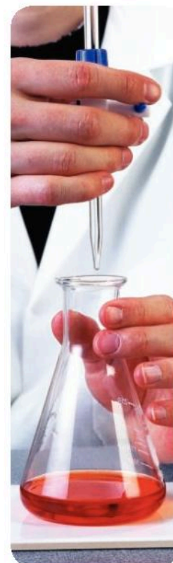
▲ The colour of the solution has changed: the titration is complete.
