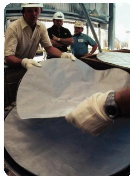
▲ A catalyst of platinum and rhodium, in the form of a gauze, is being fitted into a tank. It will catalyse the production of nitric acid from ammonia and oxygen.
