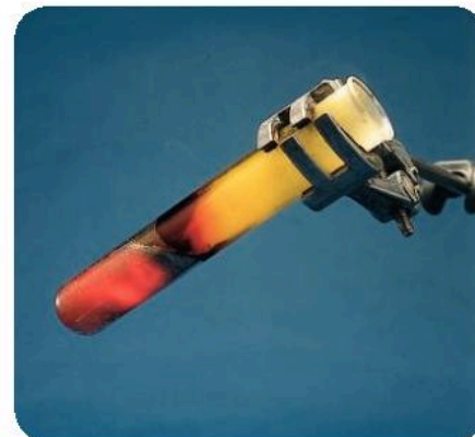
▲ Iron filings reacting with sulfur. You need heat to start the reaction off – but then it gives out heat.
