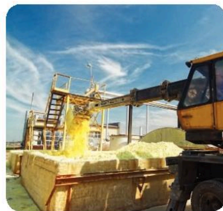
▲ This sulfur was obtained from sulfur compounds removed from natural gas.
