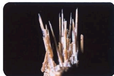
▲ If you heat rhombic sulfur slowly to above 96°C, the molecules rearrange themselves. The result is needle-shaped crystals of monoclinic sulfur.
