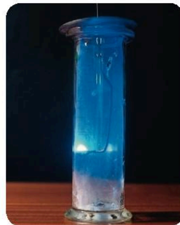
▲ Sulfur combines with oxygen when it burns.
