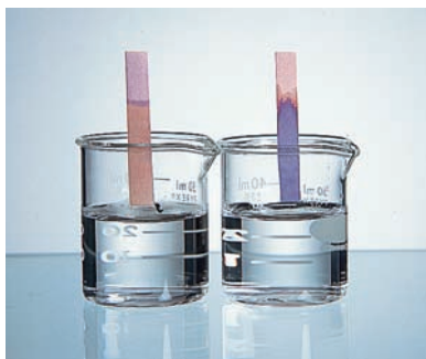
Figure 10.2 Litmus is a vegetable dye obtained from certain lichens found principally in the Netherlands. Paper treated with this dye turns from blue to red in acids (left) and from red to blue in bases (right).
