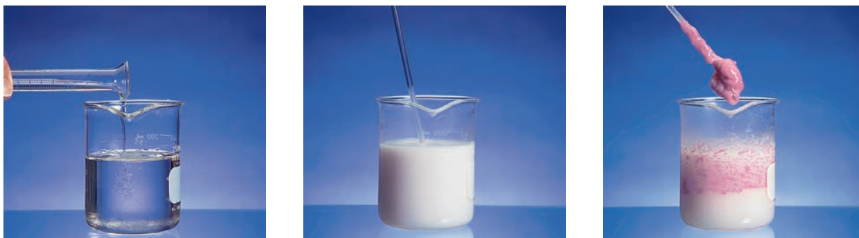
Figure 15.11 When a mixture of phenol and formaldehyde dissolved in acetic acid is treated with concentrated hydrochloric acid, a cross-linked phenol-formaldehyde network polymer is formed.
