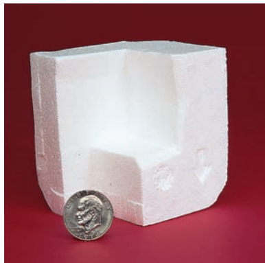
Figure 2.8 Both of these items have a mass of 23 grams, but they have very different volumes; therefore, their densities are different as well.
