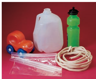
Figure 13.13 Examples of objects made of polyethylene. Polyethylene objects that are strong and rigid (bottles, toys, covering for wire) contain HDPE (high-density polyethylene). Polyethylene objects that are very flexible (plastic bags and packaging materials) contain LDPE (low-density polyethylene).
