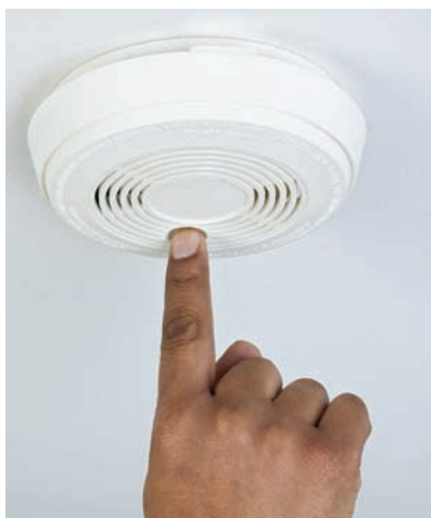
Figure 11.5 The synthetic element americium (element 95) is a component of nearly all standard smoke detectors. Small amounts of Am-241, which has a half-life of 458 years, produces radiation that ionizes air within the detector, causing it to conduct electricity. The presence of smoke in the detector causes a drop in electrical conductivity, and the alarm sounds.
