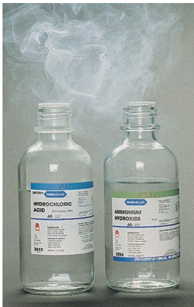
Figure 10.3 A white cloud of finely divided solid \text{NH}_4\text{Cl} is produced by the acid-base reaction that results when the colorless gases \text{HCl} and \text{NH}_3 mix. (The gases escaped from the concentrated solutions of \text{HCl} and \text{NH}_3 .)
