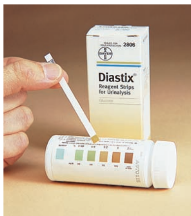
Figure 18.18 The glucose content of urine can be determined by dipping a plastic strip treated with oxidizing agents into the urine sample and comparing the color change of the strip to a color chart that indicates glucose concentration.
