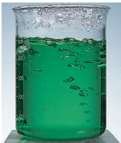
Figure 7.18 Bubbles of vapor form within a liquid when the temperature of the liquid reaches the liquid's boiling point.
