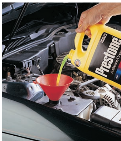
Figure 8.12 A water-antifreeze mixture has a higher boiling point and a lower freezing point than pure water.
