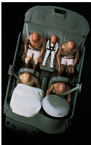
Figure 6.10 Testing apparatus for measuring the effects of airbag deployment.
