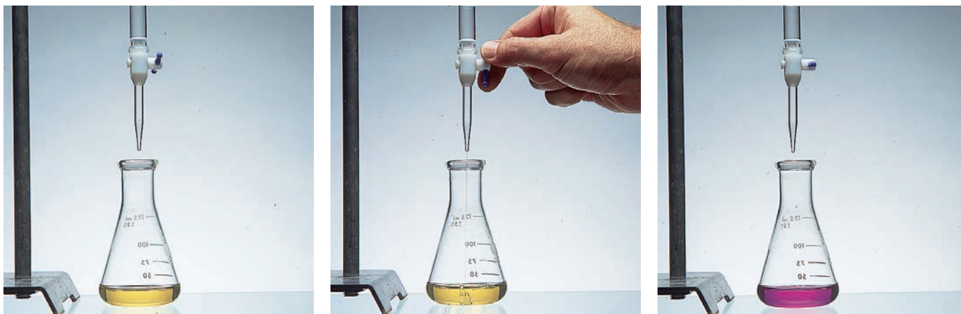
Figure 10.17 An acid–base titration using an indicator that is yellow in acidic solution and red in basic solution.
