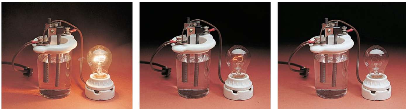
Figure 10.15 This simple device can be used to distinguish among strong electrolytes, weak electrolytes, and nonelectrolytes. The light bulb glows strongly for strong electrolytes (left), weakly for weak electrolytes (center), and not at all for nonelectrolytes (right).
