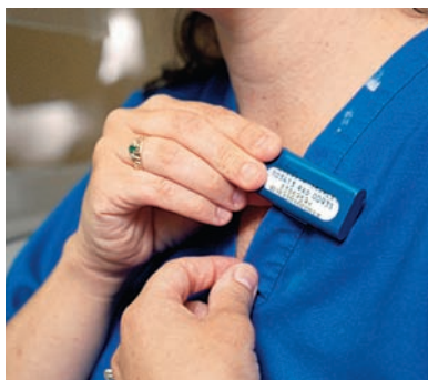
Figure 11.9 Film badges, such as the one worn by this technician, are used to determine a person's exposure to radiation.
