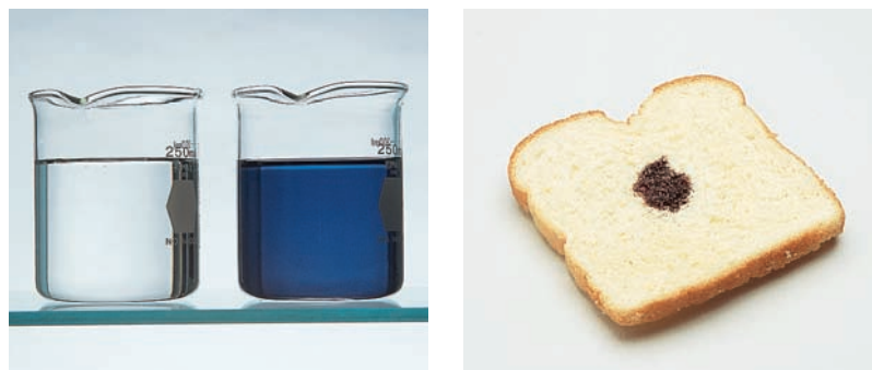
Figure 18.24 Use of iodine to test for starch. Starch-containing solutions and foods turn dark blue-black when iodine is added.
