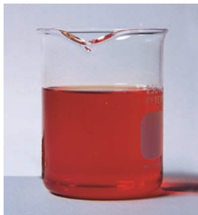
Figure 13.9 A bromine in water solution is reddish brown (left). When a small amount of such a solution is added to an unsaturated hydrocarbon, the added solution is decolorized as the bromine adds to the hydrocarbon to form colorless dibromo compounds (right).
