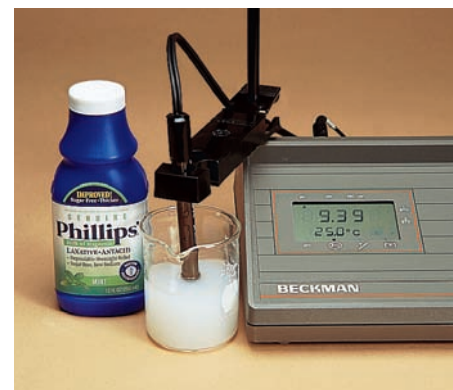
Figure 10.13 A pH meter gives an accurate measurement of pH values. The pH of vinegar is 2.32 (left). The pH of milk of magnesia in water is 9.39 (right).
