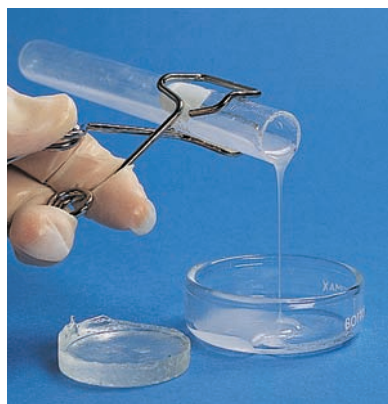
Figure 13.11 Preparation of polystyrene. When styrene, \text{C}_6\text{H}_5\text{---CH}=\text{CH}_2 , is heated with a catalyst (benzoyl peroxide), it yields a viscous liquid. After some time, this liquid sets to a hard plastic (sample shown at left).
