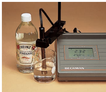
Figure 10.13 A pH meter gives an accurate measurement of pH values. The pH of vinegar is 2.32 (left). The pH of milk of magnesia in water is 9.39 (right).
