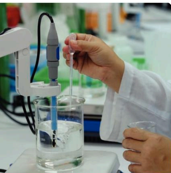
▲ Changes in pH can be monitored using a pH probe
