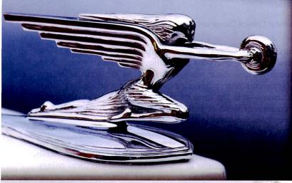
**Plating It On** Electroplating chromium onto this 1936 Packard hood ornament, both for beauty and protection against corrosion, requires energy. The other face of electrochemistry is represented by batteries, which supply energy. This chapter will reveal both faces.
