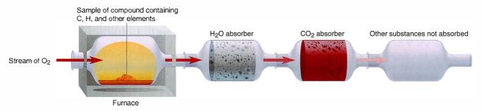
Figure 3.5 Combustion apparatus for determining formulas of organic compounds. A sample of compound that contains C and H (and perhaps other elements) is burned in a stream of  $O_2$  gas. The  $CO_2$  and  $H_2O$  formed are absorbed separately, while any other element
