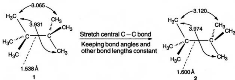
Figure 3.8. Structures for a simple MM “by hand” calculation on the effect of changing the central C–C length of (\text{CH}_3)_3\text{C}-\text{C}(\text{CH}_3)_3 from 1.538 to 1.600 Å.
