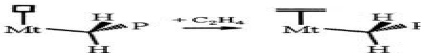
Figure 3. Modified Cossee mechanism for the polymerization of olefins with early transition metals. Green, Rooney and Brookhart introduced the presence of the adjuvant \alpha -agostic interaction in the transition state.
