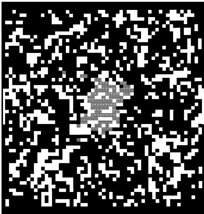
Figure 16 A model of the disruption of a crystal in water. The dark cells represent water, the white cells are cavities, and the grey cells are solute molecules.
