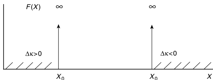
Figure 5 Upper energy ( \Delta\kappa > 0 ) and lower energy ( \Delta\kappa < 0 ) fluctuations boundaries in the Q model.
