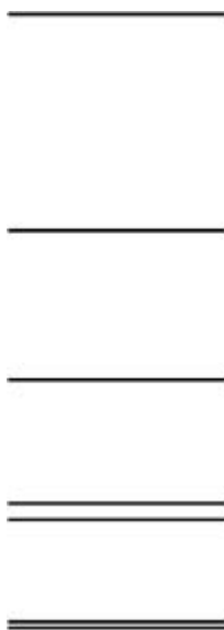
Figure A1.2.9. Energy level pattern of polyad 6 of a spectroscopic Hamiltonian for coupled stretches with strong Darling–Dennison coupling. Within the polyad the transition from normal to local modes is evident. At the bottom of the polyad are two nearly degenerate pairs of levels. Semiclassically, the bottom pair derive from local mode overtone states. The levels are symmetrized mixtures of the individual local mode overtones. Semiclassically, they are exactly degenerate; quantum mechanically, a small splitting is present, due to tunnelling. The next highest pair are symmetrized local mode combination states. The tunnelling splitting is larger than in the bottom pair; above this pair, the levels have normal mode character, as evidenced by the energy level pattern.
