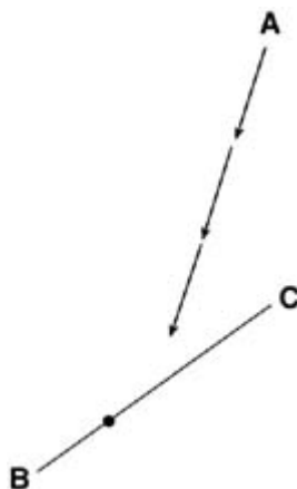
Figure B3.4.14. The infinite-order-sudden approximation for A + BC \rightarrow AB + C . In this approximation, the BC molecule does not rotate until reaction occurs.
