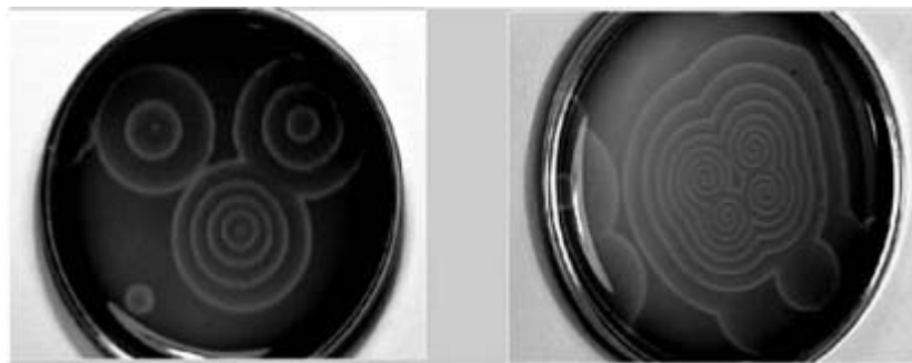
Figure A3.14.9. Reaction–diffusion structures for an excitable BZ system showing (a) target and (b) spiral waves. (Courtesy of A F Taylor.)
