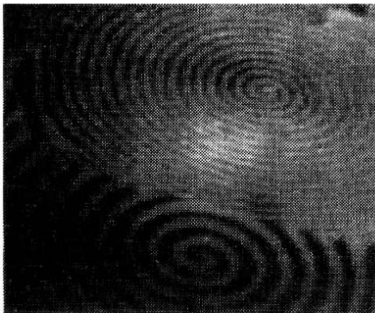
Figure A3.14.11. Spiral waves imaged by photoelectron electron microscopy for the oxidation of CO by O 2 on a Pt(110) single crystal under UHV conditions. (Reprinted with permission from [35], © The American Institute of Physics.)
