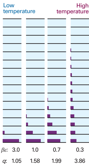
Fig. 16.6 The populations of the energy levels of the system shown in Fig. 16.3 at different temperatures, and the corresponding values of the partition function calculated in Example 16.2. Note that \beta = 1/kT .
