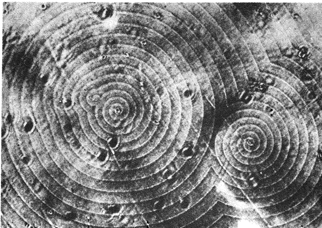
Fig. VII-9. Screw dislocation in a carborundum crystal. (From Ref. 116.)
