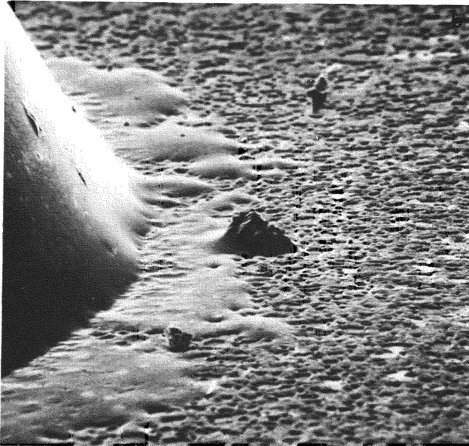
Fig. X-14. SEM picture of a drop of cooled glass on Fernico metal (which has the same coefficient of thermal expansion), \times 130 . (From Ref. 183.)
