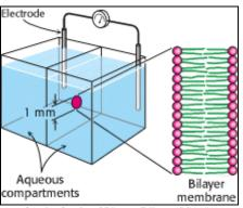
Figure 12.14. Experimental Arrangement for the Study of Planar Bilayer Membrane. A bilayer membrane is formed across a 1-mm hole in a septum that separates two aqueous compartments. This arrangement permits measurements of the permeability and electrical conductance of lipid bilayers.
