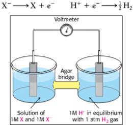
Figure 18.6. Measurement of Redox Potential. Apparatus for the measurement of the standard oxidation-reduction potential of a redox couple. Electrons, but not X or X<sup>-</sup>, can flow through the agar bridge.
