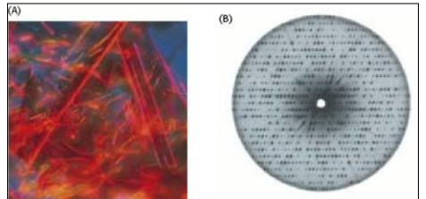
Figure 4.51. Myoglobin Crystal and X-Ray. (A) Crystal of myoglobin. (B) X-ray precession photograph of a myoglobin crystal. [(A) Mel Pollinger/Fran Heyl Associates.]
