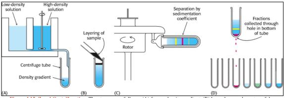
**Figure 4.15. Zonal Centrifugation.** The steps are as follows: (A) form a density gradient, (B) layer the sample on top of the gradient, (C) place the tube in a swinging-bucket rotor and centrifuge it, and (D) collect the samples. [After D. Freifelder, *Physical Biochemistry*, 2d ed. (W. H. Freeman and Company, 1982), p. 397.]
