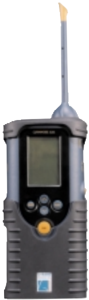
FIGURE 32.9 The Cyranose 320. The electronic nose may find uses in the food industry, animal husbandry, law enforcement, and medicine. [Courtesy of Cyrano Sciences.]
