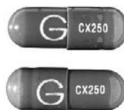
Figure 12.8 Examples of capsule showing marking reversed on cap and body. (Courtesy of TICTAC Communications Ltd.)
