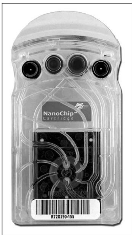
Figure 22.9 The NanoChip Cartridge, which is used with a NanoChip Molecular Biology Workstation. Electrical charges guide DNA samples down microfluidic channels to the NanoChip Microelectronic Array (see Fig. 22.10), which enables the precise identification of active genes. (Courtesy of Nanogen.)
