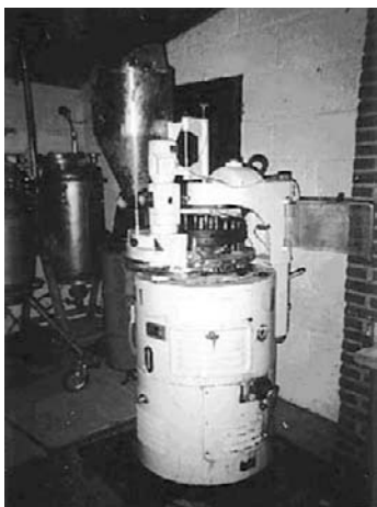
Figure 12.3 Commercial tablet machine used to produce illicit tablets. (Courtesy of TICTAC Communications Ltd.)
