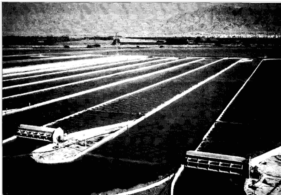
Figure 7.2 Production-scale ponds for the culture of the halophilic green alga Dunaliella . This organism is grown by the Japanese company NBT (Nature Beta Carotene) on the shores of the Gulf of Eilat, Northern Red Sea in Israel. The algae are harvested by centrifugation and dried, and then sold as a food supplement rich in \beta -carotene, mostly the essential 9- cis isomer.
