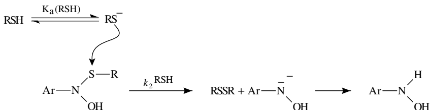
SCHEME 3. Mechanism of N -hydroxyarylamine formation (from Kazanis and McClelland 30 , with modification)
