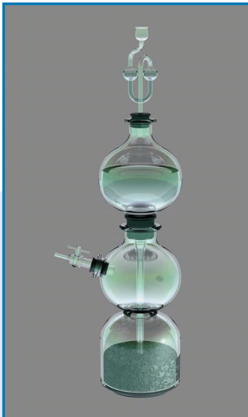
Figure 5.1 Made with three connected glass bowls, Kipp's apparatus relies on acid-base chemistry in order to produce gasses—such as carbon dioxide, hydrogen, or hydrogen sulfide—for chemists to use in other chemical reactions.
