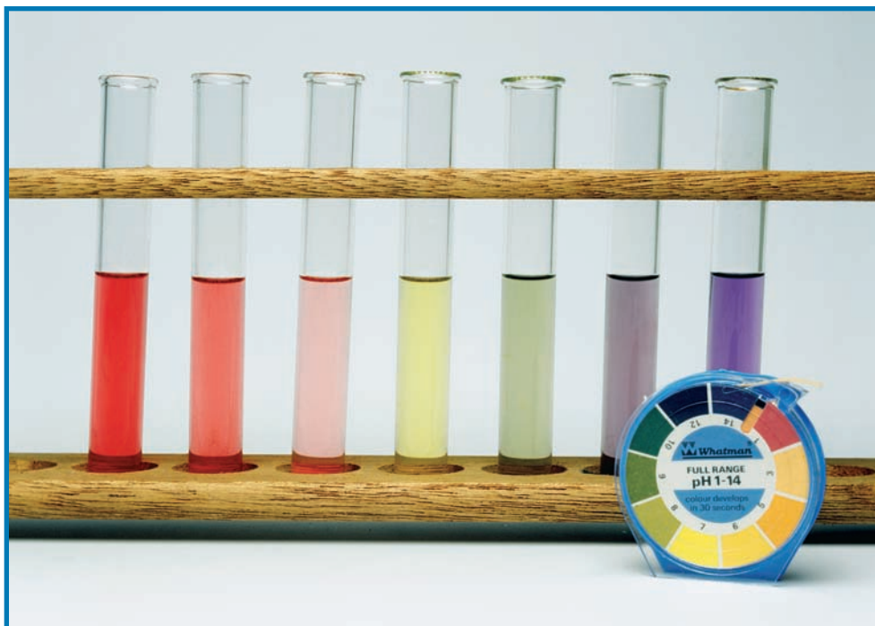
Figure 3.4 An acid-base indicator called universal indicator can show the exact pH of a substance. Adding a small amount of universal indicator to a solution changes the color of the solution. Each color represents a different pH.
