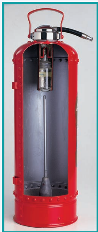
Figure 4.1 In a soda-acid fire extinguisher, a chemical reaction between an acid (sulfuric acid) and a base (baking soda) produces a jet of water that can put out certain kinds of fires.
