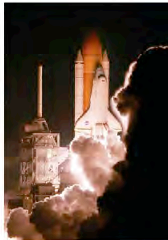
FIGURE 1.3 Hydrogen reacts with oxygen, producing water and releasing energy. Energy from this reaction propels the U.S. space shuttles. During liftoff, each of the five main engines of the shuttle consumes about 40 tons per minute of hydrogen and oxygen, which are stored in the large brown tank under the shuttle. Once in space, the electric power needs of the space shuttles are supplied by fuel cells energized by the same chemical reaction between hydrogen and oxygen. The water generated as a product of this reaction is used aboard the shuttle.
