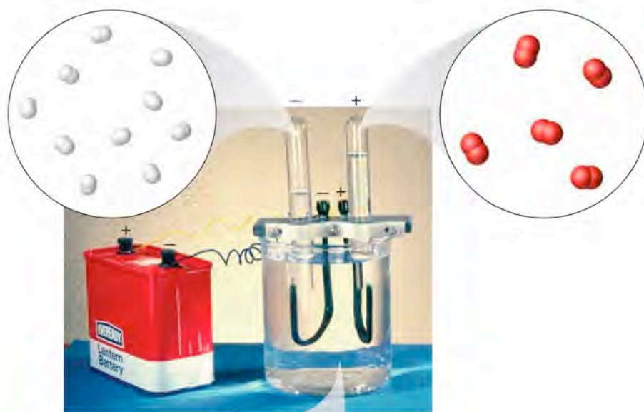
FIGURE 1.3 Hydrogen reacts with oxygen, producing water and releasing energy. Energy from this reaction propels the U.S. space shuttles. During liftoff, each of the five main engines of the shuttle consumes about 40 tons per minute of hydrogen and oxygen, which are stored in the large brown tank under the shuttle. Once in space, the electric power needs of the space shuttles are supplied by fuel cells energized by the same chemical reaction between hydrogen and oxygen. The water generated as a product of this reaction is used aboard the shuttle.
