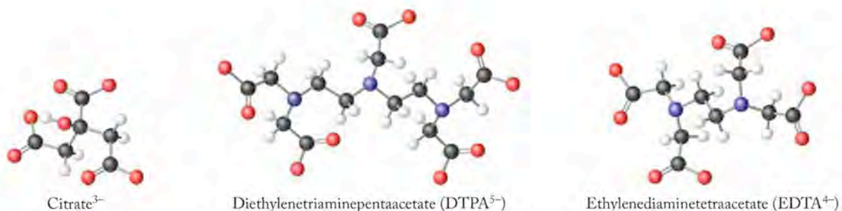
FIGURE 21.12 Citrate 3- , diethylenetriaminepentaacetate (DTPA 5- ), and ethylenediaminetetraacetate (EDTA 4- ) are often used as chelating agents in diagnostic and therapeutic agents based on transition metals. They form stable complex ions with 2+ and 3+ metal cations. Citrate, DTPA, and EDTA complexes are also more soluble than simple binary salts.
