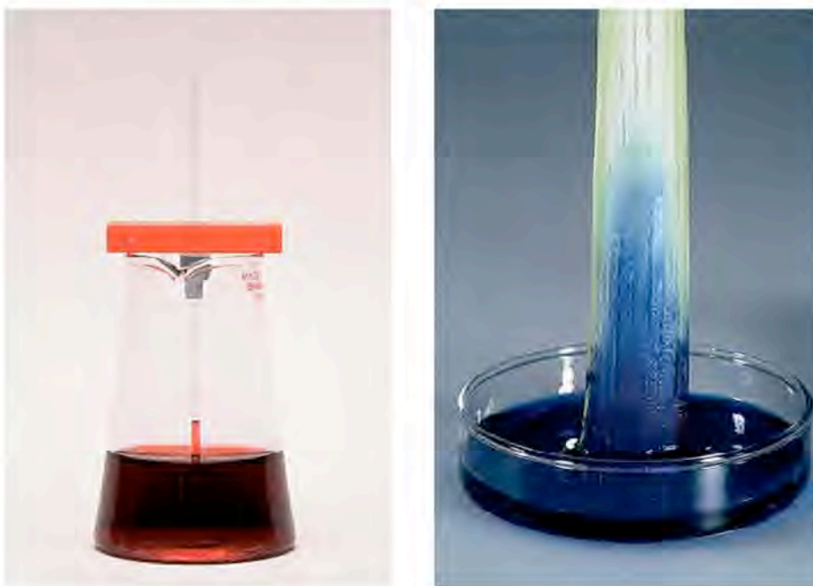
FIGURE 10.21 Water rises in a thin glass capillary tube and also in a stick of celery because of capillary action.
