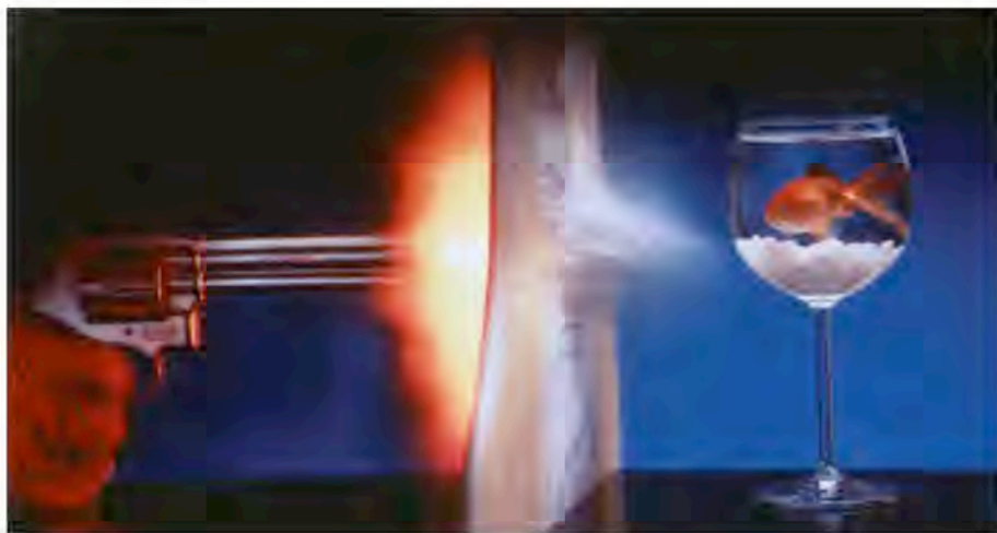
FIGURE 12.25 Illustration of the strength of Kevlar: a bullet fired point-blank at a sheet of Kevlar does not puncture the fabric.
