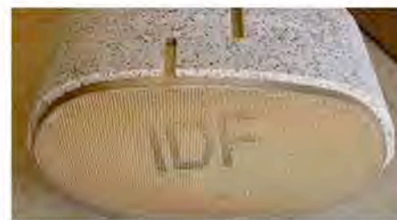
FIGURE 14.27 Catalytic converters. (a) In an automobile the converter is located close to the engine because it works best at high temperatures before gases have a chance to cool. (b) The structure of a catalytic converter. (c) The porous ceramic honeycomb support for the metal catalysts.
