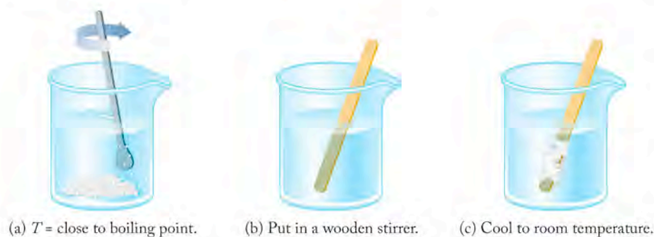
FIGURE 4.10 Making rock candy: (a) Sugar is very soluble in hot water; (b) as a hot, saturated solution of sugar in water cools, (c) the solute gradually precipitates.
