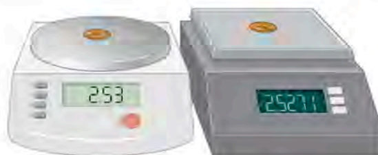
FIGURE 1.15 The mass of a penny can be measured to the nearest 0.01 gram with the balance on the left, and to the nearest 0.0001 gram with the balance on the right.
