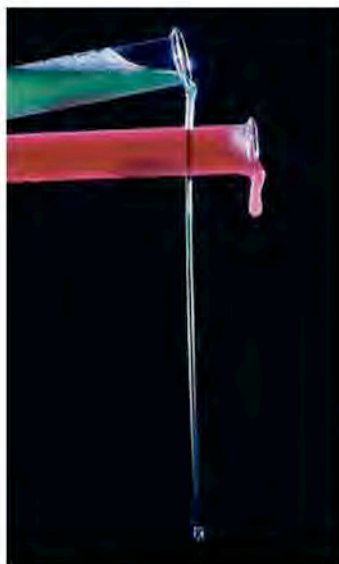
FIGURE 10.22 High viscosity results from strong intermolecular forces between large polar molecules. The red fluid is more viscous than the green, which pours freely.
