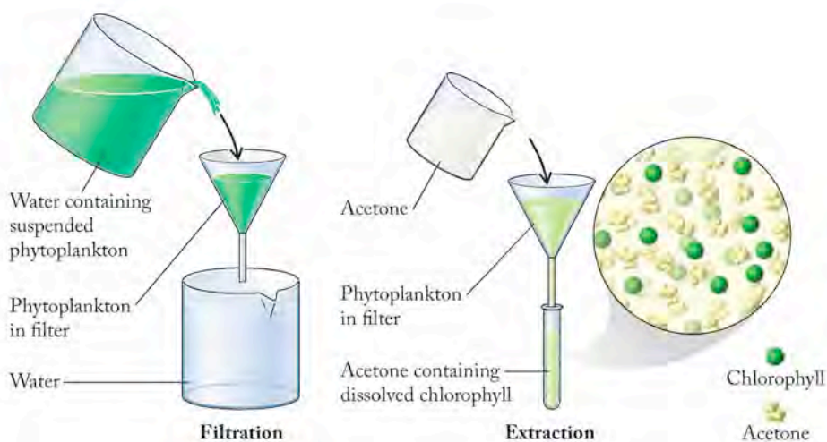
FIGURE 4.5 Particles in suspension, such as phytoplankton in seawater, can be separated by filtration. Scientists may extract the material trapped on the filter with an organic solvent such as acetone that dissolves the phytoplankton's chlorophyll and other pigments. The intensity of the color of these acetone extracts provides a measure of the concentration of phytoplankton in the original sample.
