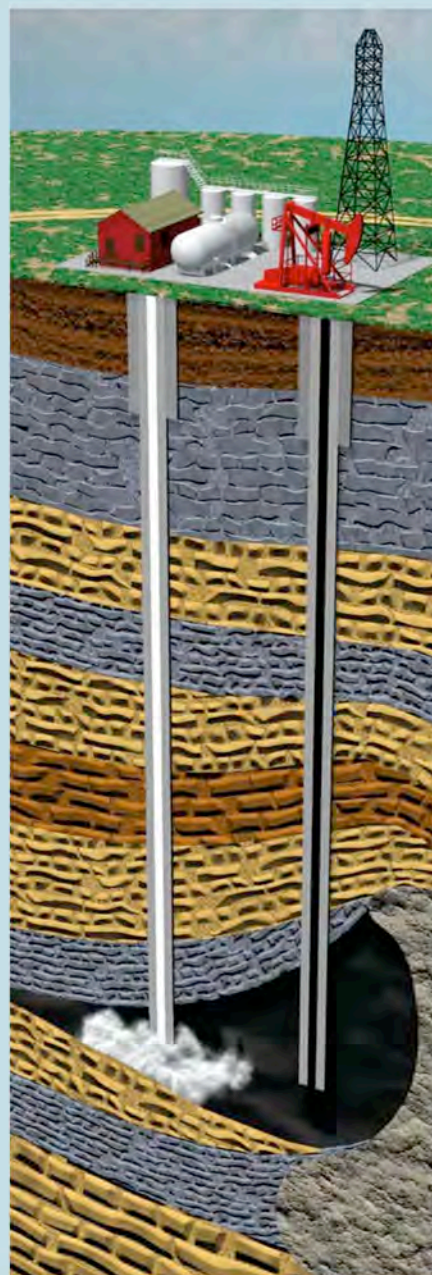
FIGURE 6.30 Nitrogen under high pressure is pumped into oil deposits to bring crude oil to the surface.
