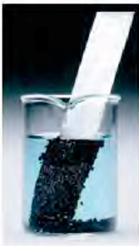
FIGURE 18.1 A strip of zinc immersed in a solution of copper(II) sulfate becomes encrusted with a dark layer of copper. The blue color of the solution fades as \text{Cu}^{2+} ions (the source of the color) are reduced to Cu metal, and Zn metal is oxidized to colorless \text{Zn}^{2+} ions.
