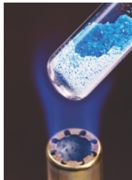
▲ FIGURE 14.13 Blue crystals of \text{CuSO}_4 \cdot 5 \text{H}_2\text{O} are converted to white anhydrous \text{CuSO}_4 when the sample is heated with a Bunsen flame.
