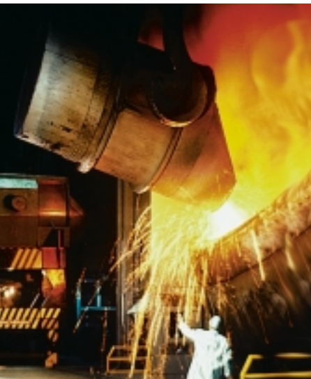
▲ Using the basic oxygen process to make steel.
