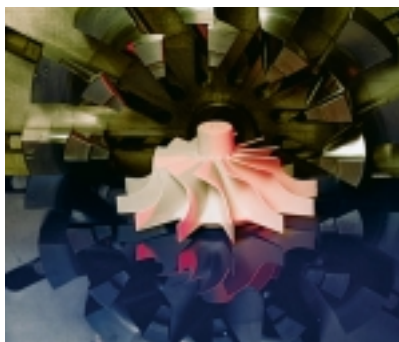
▲ A silicon nitride rotor for use in gas-turbine engines.
