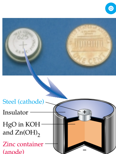
▲ FIGURE 18.10 A small mercury battery and a cutaway view.
