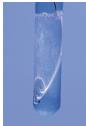
▲ Magnesium metal reacts with aqueous acid to give bubbles of hydrogen gas and \text{Mg}^{2+} ion.
