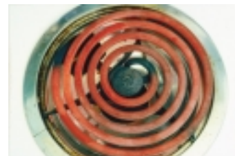
▲ The red glow given off by the heating element is an example of blackbody radiation.
