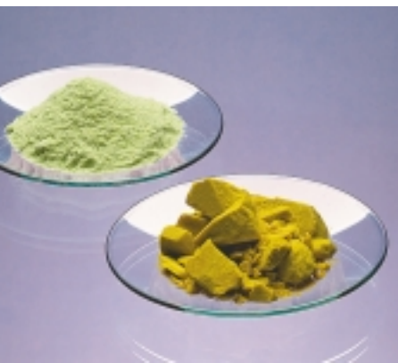
▲ Crystals of iron(II) chloride tetrahydrate are greenish; crystals of iron(III) chloride hexahydrate are brownish yellow.
