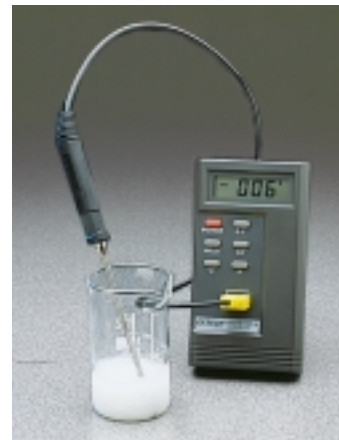
▲ FIGURE 8.6 The reaction of barium hydroxide octahydrate with ammonium chloride is so strongly endothermic and draws so much heat from the surroundings that the temperature falls below 0^\circ\text{C} and moisture freezes around the container.
