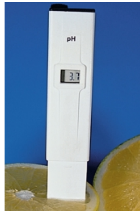
▲ FIGURE 15.6 A pH meter with its electrical probe dipping into a grapefruit. An accurate value of the pH (3.7) is shown on the meter.
