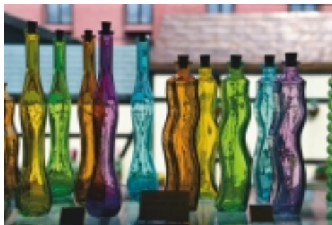
▲ Colored glasses contain transition metal ions; borosilicate glass is used in cooking utensils because of its resistance to thermal shock.
