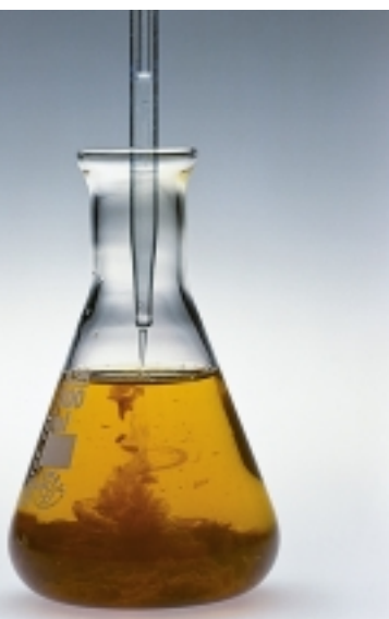
▲ FIGURE 20.10 When dilute NaOH is added to a solution of iron(III) sulfate, \text{Fe}_2(\text{SO}_4)_3 , a gelatinous, red-brown precipitate of \text{Fe}(\text{OH})_3 forms.
