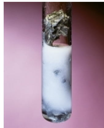
▲ Zinc metal reacts with aqueous hydrochloric acid to give hydrogen gas and aqueous \text{Zn}^{2+} ions.
