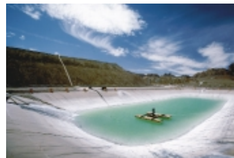
▲ A cyanide leaching pool for extracting gold at the Picacho Gold Mine in the Mohave Desert.
