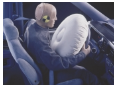
▲ Automobile air bags are inflated with \text{N}_2 gas produced by decomposition of sodium azide.
