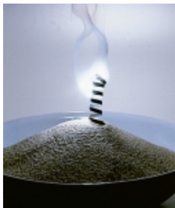
▲ Magnesium metal burns in air to give MgO.
