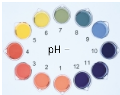
▲ FIGURE 15.5 (a) The color of universal indicator in solutions of known pH from 1 to 12. (b) The color of universal indicator in some familiar products gives the following approximate pH values: vinegar, pH 3; club soda, pH 4–5; household ammonia, pH \geq 10.
