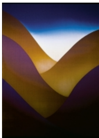
▲ The iridescent colors on this piece of metal are produced by anodizing different parts of the surface at different voltages.
