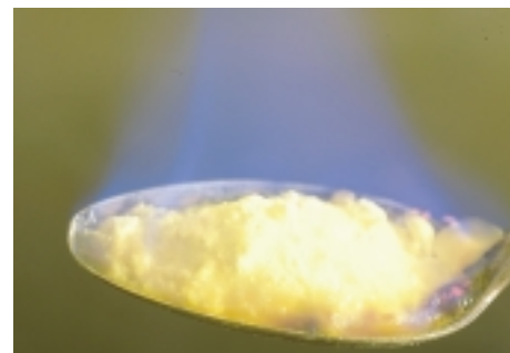
▲ Sulfur burns with a bluish flame to yield colorless SO 2 gas.
