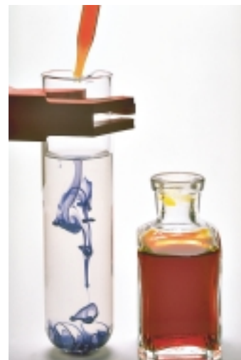
▲ The red \text{I}_3^- solution turns a deep blue color when it is added to a solution containing a small amount of starch.
