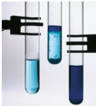
▲ FIGURE 20.11 When an aqueous solution of \text{CuSO}_4 (left) is treated with aqueous ammonia, a blue precipitate of \text{Cu}(\text{OH})_2 forms (center). On the addition of excess ammonia, the precipitate dissolves, yielding the deep blue \text{Cu}(\text{NH}_3)_4^{2+} ion (right).
