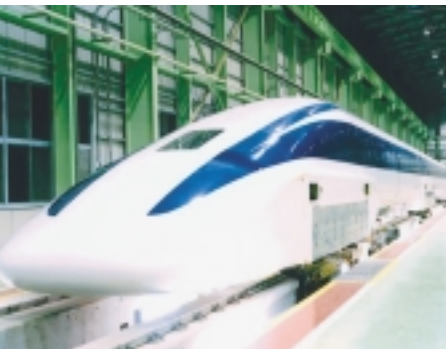
▲ FIGURE 21.15 An experimental magnetically levitated train (Maglev) in Japan is suspended above superconducting magnets that are cooled with liquid helium. This five-car train has attained a speed of 552 km/h in a manned vehicle run.
