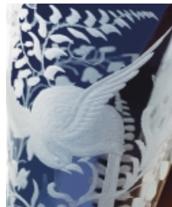
▲ Gaseous HF is one of the few substances that reacts with and etches glass ( \text{SiO}_2 ), according to the equation \text{SiO}_2(\text{s}) + 4 \text{HF}(\text{g}) \rightarrow \text{SiF}_4(\text{g}) + 2 \text{H}_2\text{O}(\text{l}) .
