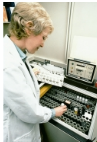
▲ Radiation is conveniently detected and measured using this scintillation counter, which electronically counts the flashes produced when radiation strikes a phosphor.
