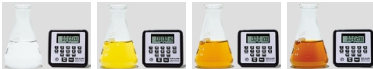
▼ FIGURE 12.5 A sequence of photographs showing the progress of the reaction of hydrogen peroxide ( \text{H}_2\text{O}_2 ) and iodide ion ( \text{I}^- ). As time passes (left to right), the red color due to triiodide ion ( \text{I}_3^- ) increases in intensity.
