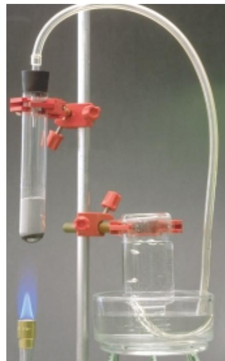
▲ \text{MnO}_2 catalyzes the thermal decomposition of \text{KClO}_3 to \text{KCl} and \text{O}_2 gas.
