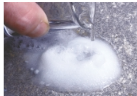
▲ Carbonate-bearing rocks like limestone ( \text{CaCO}_3 ) react with dilute acids such as HCl to produce bubbles of carbon dioxide.
