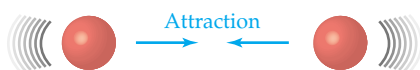
▲ FIGURE 9.15 Molecules attract one another at distances up to about 10 molecular diameters. The result is a decrease in the actual volume of most real gases when compared with ideal gases at pressures up to 300 atm.
