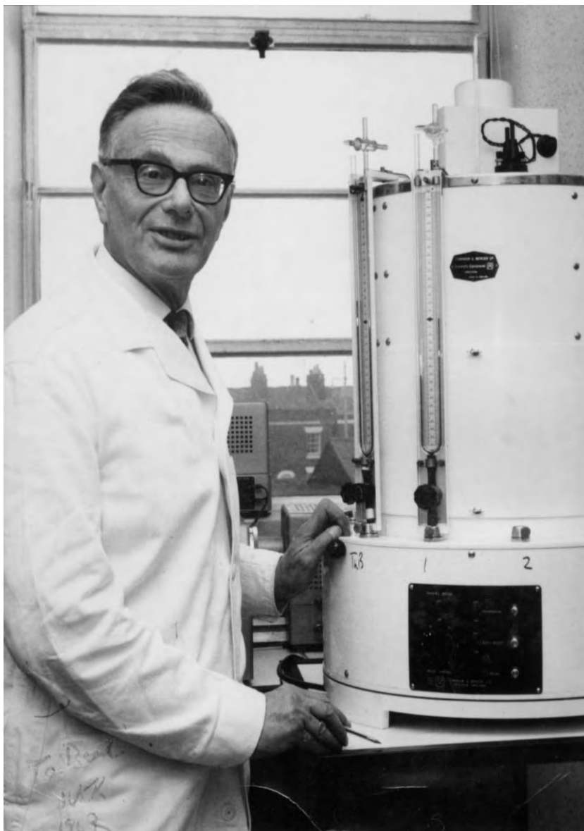
FIGURE 1 Hans Krebs at age 68 in his laboratory at Oxford standing next to his beloved Warburg apparatus, which he learned to use in the laboratory of Otto Warburg and which was the major instrument used in his discovery of both the urea and the citric acid cycles. The square box in the background is a power supply for a Zeiss PMQ spectrophotometer. The spectrophotometer was first devised by Otto Warburg who also first discovered pyridine nucleotide and observed their spectral shift during oxidation/reduction. This spectral change formed the basis of many of the assays Krebs undertook in his later years. With these simple instruments and a devoted staff he worked happily in this building at the Radcliffe Infirmary until he was 81, when he died in a hospital ward in the same building in 1981 after a 2 week illness.
