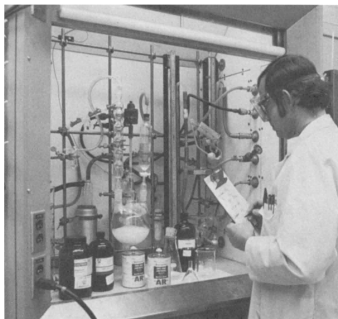
Fig. 3. Typical laboratory apparatus showing preparation of 2-phenyl-2-decanol by a Grignard reaction. (The Dow Chemical Company)
