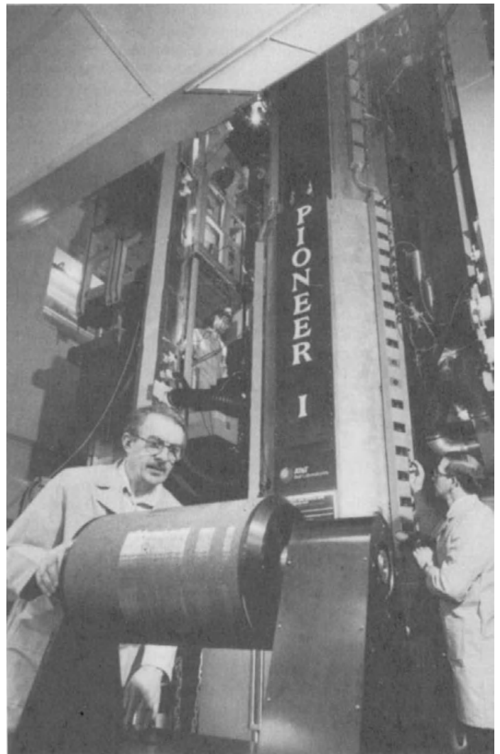
Fig. 4. Experimental optical fiber designs are tested by creating glass preforms, heating them in a special furnace located above the research fiber drawing tower (as shown) and drawing the fiber from the preform onto a collection drum shown in the foreground. The fiber is then used in tests conducted with light generators (lasers and LEDs) and photodetectors. The single-mode fiber is rated for high-capacity transmission, while lower-capacity multimode fibers are well matched to various economical sources and detectors. (AT&T Bell Laboratories)
