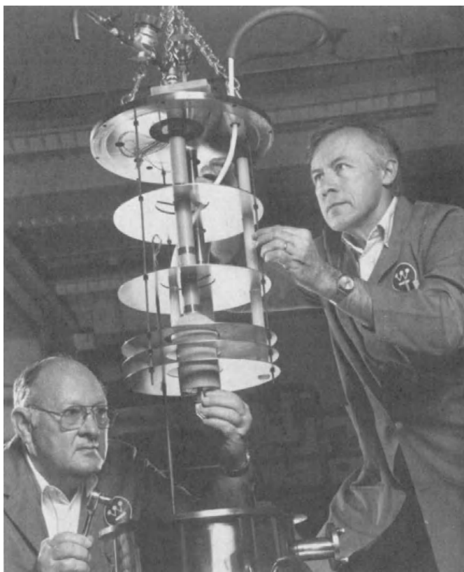
Fig. 2. Electrical lead comprised of a high-temperature superconductor can carry a current of 2000 amperes. A variety of uses include magnetic resonance imaging and superconducting magnetic energy storage. (Westinghouse Electric Corporation)
