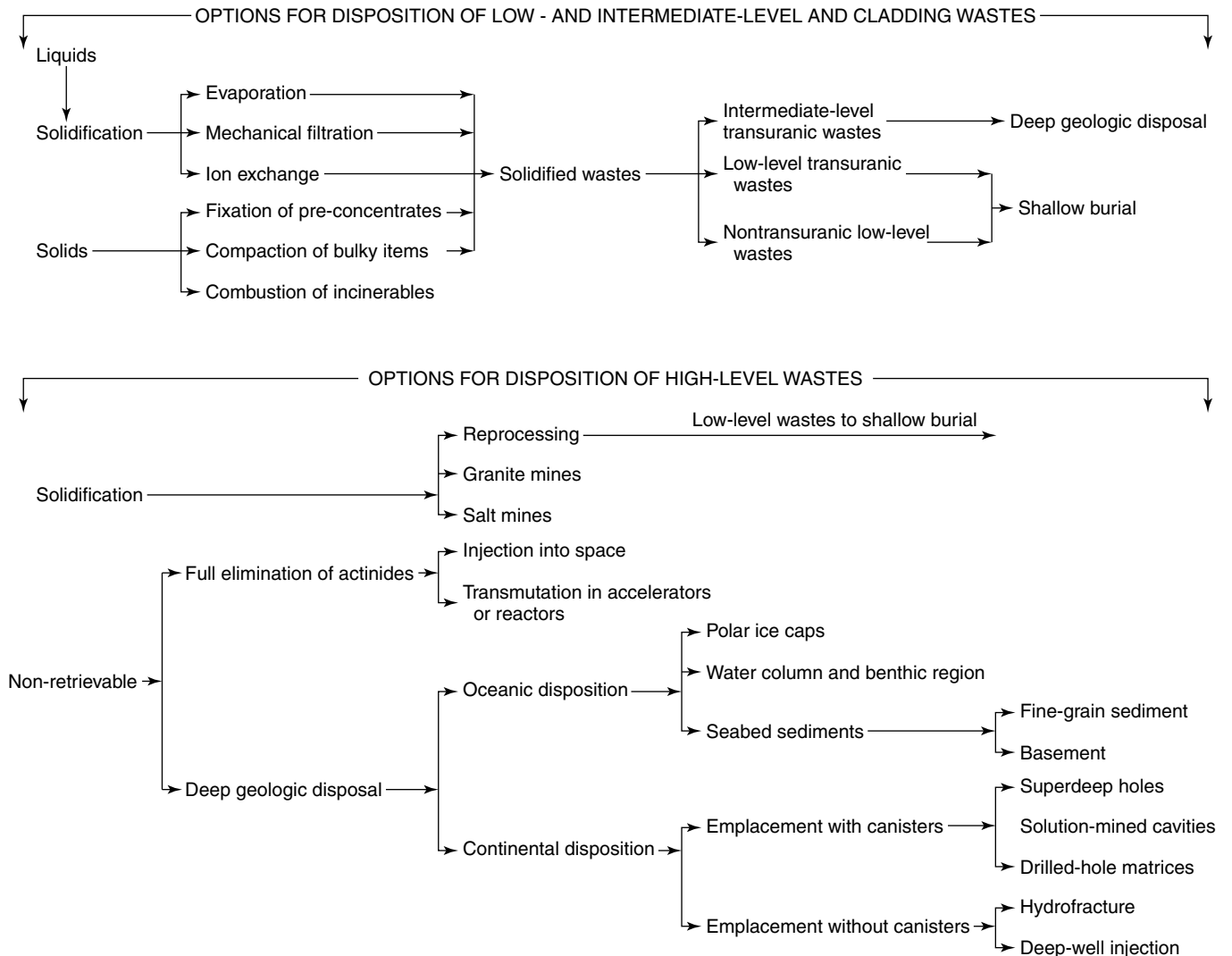
Fig. 39. Panorama of options for consideration in the disposition of radioactive wastes. (Top portion of chart: Options for disposition of low- and intermediate-level and cladding wastes. Bottom portion of chart: Options for disposition of high-level wastes)
