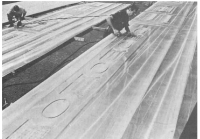
Fig. 3. Final operations on machined aluminum plates for wings of large jet aircraft. (Reynolds Metals Company.)
