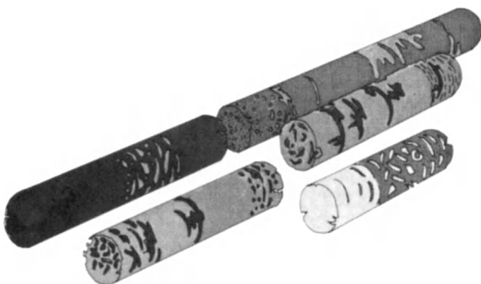
Fig. 13. Rock core samples cut by a diamond-faced core bit reveal underlying structure and the possible presence of hydrocarbons. (Exxon Corp)
