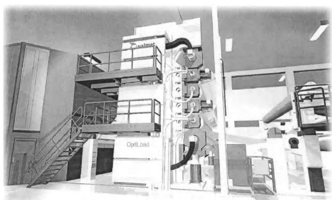
Fig. 7. Multipip calender as part of paper machine. (Valmet Corporation)
