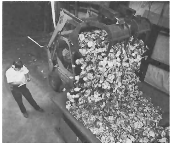
Fig. 2. Recycling of aluminum beverage cans and other scrap saves nearly 95% of the energy required when producing the virgin metal from ore. Approximately 50% of the metal processed in 1990 was recycled from scrap. (Reynolds Aluminum Recycling Company)
