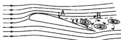
Fig. 5. Partial burble on airfoil at high angle of attack: (A) stagnation point; (B) line of separation
