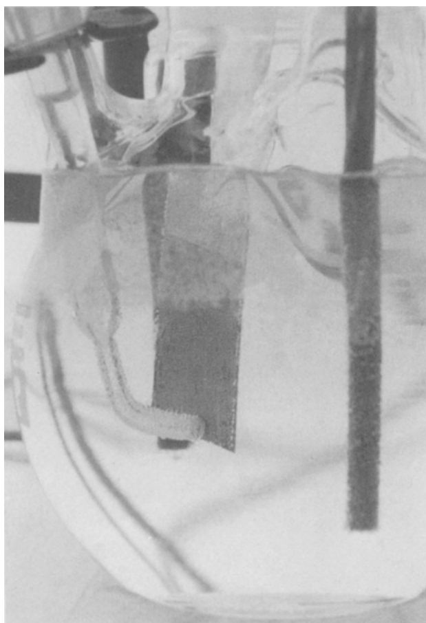
Fig. 1. Apparatus for testing corrosion of metal coated with a plastic. ( The Dow Chemical Company )
