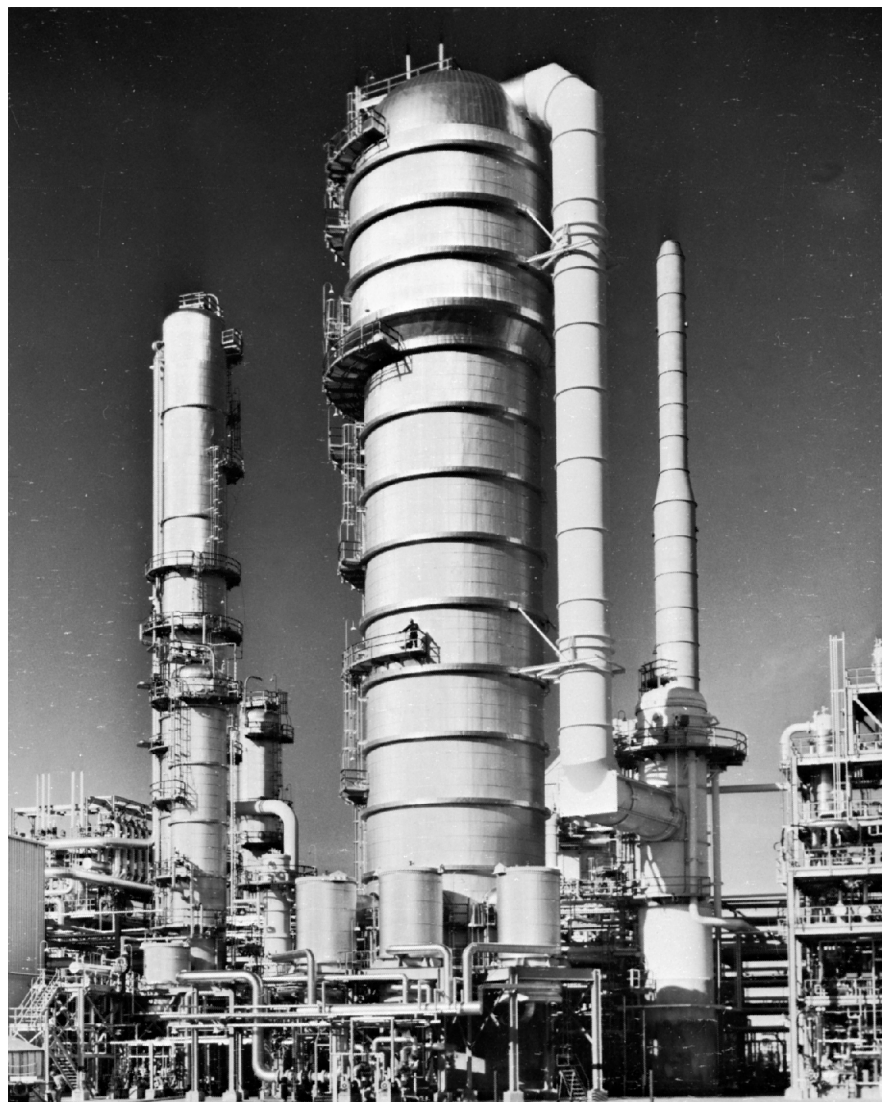
FIGURE 1 Large distillation column for the production of styrene. [Courtesy of Shell Chemical Canada, Ltd.]
