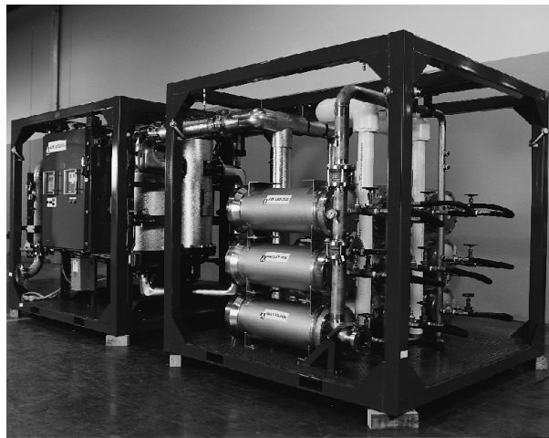
FIGURE 17 Compact nitrogen enrichment membrane system. (Courtesy Air Liquide.)
