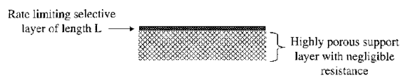
FIGURE 2 Idealized high-performance synthetic membrane showing a top rate-limiting selective layer and an "invisible" (with regard to transport) supporting layer.
