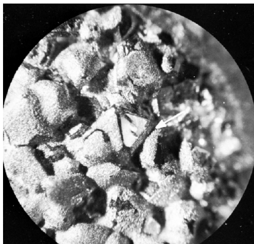
FIGURE 9 Freshly grown diamonds bearing a thin film of nickel. The arrow indicates a bare octahedral face about 0.1 mm in size.
