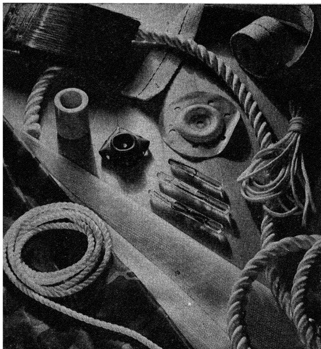
FIG. 183.—Nylon's uses have been extended far beyond hosiery, tooth-brush bristles, and tennis racket strings since the war began. Arranged clockwise, beginning at the paintbrush with tapered bristles, are parachute harness webbing, parachute shroud lines, rope for military gliders, cargo parachute cloth, camouflaged Army Air Force escape parachute cloth, and light rope. In the center are experimental molded plastic bearing, carburetor diaphragms, and surgical sutures. (Courtesy of E. I. du Pont de Nemours & Company, Inc.)
