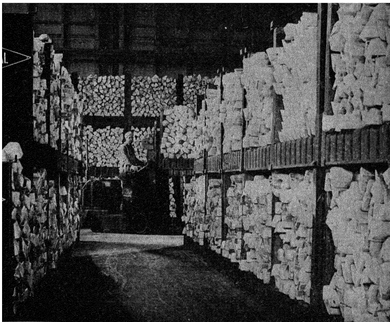
FIG. 152.—Magnesium ingots in storage. (Courtesy of the Dow Chemical Company.)
