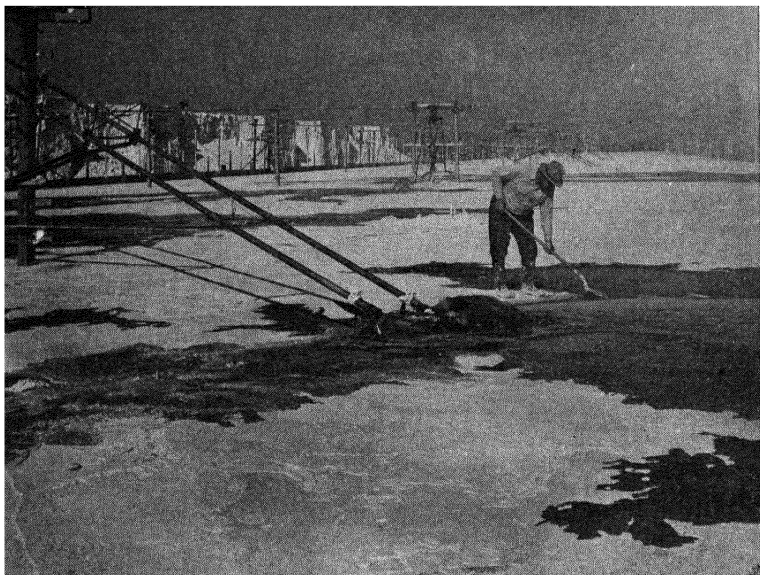
FIG. 115.—Liquid sulfur pouring into a storage vat. (Courtesy of Texas Gulf Sulphur Company.)
