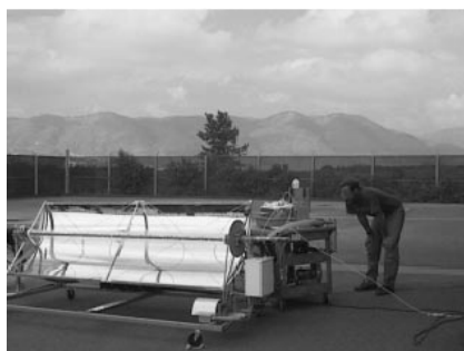
Figure 22.4.2. Schematic of the 10 SCFM parabolic trough, solar photoreactor system used at Fort Carson U. S. Army Installation.
