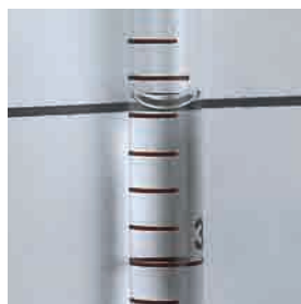
Figure F.4 A meniscus reader helps you read the volume of liquid more easily
