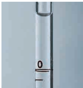
Figure F.1 Draw a bit more liquid than you need into the pipette. It is easier to reduce this volume than it is to add more solution to the pipette.
