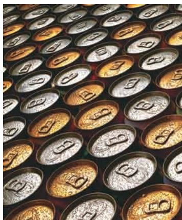
Figure 11.24 The alloy used to make pop cans contains about 97% aluminum, by mass. The other elements in the alloy are magnesium, manganese, iron, silicon, and copper.
