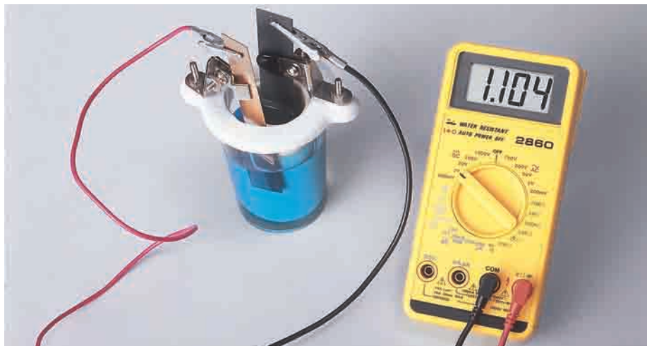
Figure 11.1 The Daniell cell is named after its inventor, the English chemist John Frederic Daniell (1790–1845). In the photograph shown here, the zinc sulfate solution is placed inside a porous cup, which is placed in a larger container of copper sulfate solution. The cup acts as the porous barrier.
