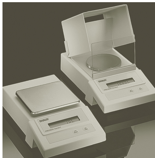
Figure 1.2 Two balances with different sensitivities
