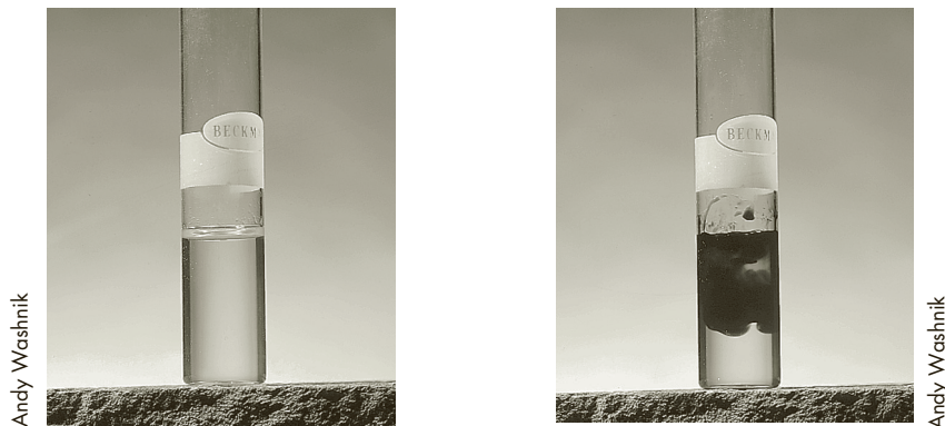
Figure 29.1 I_3^- without starch added (left); I_3^- with starch added (right)
