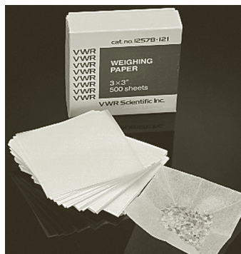
Figure 29.3 Weighing paper for measuring the \text{KIO}_3 primary standard
