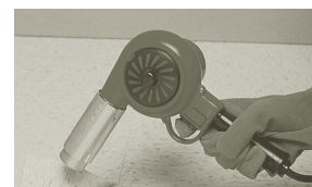
Figure 4.7 A low temperature heat gun can accelerate the drying.
