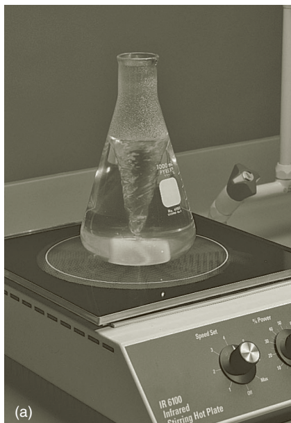
Figure 20.3 Gently heat the sample to remove \text{CO}_2(\text{g}) .
