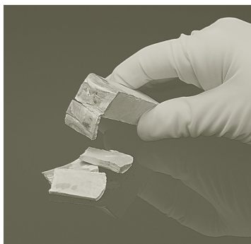
Sodium metal is a shiny, but very reactive metal, typical of Group 1A elements.
