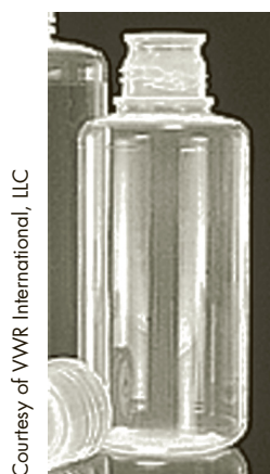
Figure 9.2 A 500-mL polyethylene bottle for the NaOH solution
