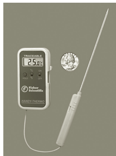
Figure 25.3 A modern digital thermometer can be substituted for a glass thermometer.
