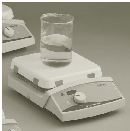
Figure T.13a A hot plate may be used to maintain solutions in a beaker or flask at a constant, elevated temperature for an extended time period.
