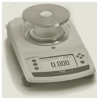
Figure T.6a Top-loading balance, sensitivity of \pm 0.01 g and/or \pm 0.001 g.
