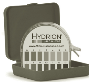
Figure 6.6 The pH of a solution can be estimated with pH paper, such as Hydrion® pH test paper, a strip of paper that is impregnated with a mixture of acid–base indicators. A gradation of colors on the pH paper approximates the pH of the solution.
