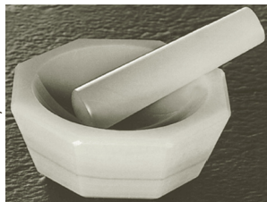
Figure 30.3 A mortar and pestle is used to grind the sample
