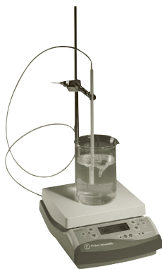
Figure 26.3 A stirring hot plate with a thermal sensor can be used to set water bath temperatures.
