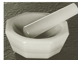
Figure 29.5 A mortar and pestle is used to grind the powder.
