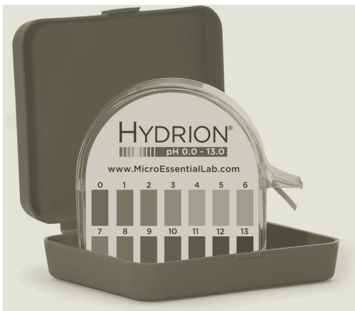
Figure T.17c Hydrion® pH test papers impregnated with a mixture of acid–base indicators can be used to measure the approximate pH of a solution.
