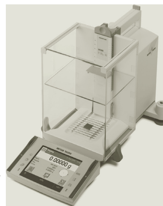
Figure T.6c Analytical balance, sensitivity of \pm 0.00001 g.
