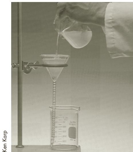
Figure 8.2 Gravity filtration is used to filter finely divided precipitates.
