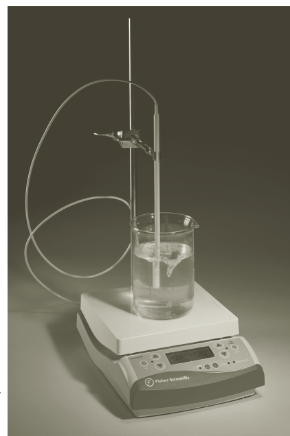
Figure T.13b A stirring hot plate may be used to heat a liquid and minimize “bumping.”
