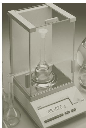
Figure T.6b Analytical balance, sensitivity of \pm 0.0001 g.
