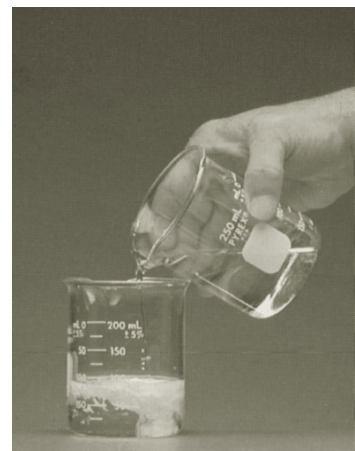
Figure 16.2 Solid AgCl quickly forms when solutions containing Ag + and Cl - are mixed.
