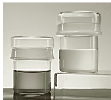
The \text{Cu}^{2+} ion in solution (right) has a less intense color than does the deep-blue [\text{Cu}(\text{NH}_3)_4]^{2+} complex.
