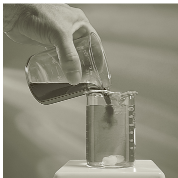
Figure 27.3 The deep purple permanganate ion, added to an acidic iron(II) solution, is reduced to the nearly colorless manganese(III) ion.
