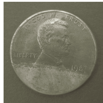
Figure 28.1 The penny is made of zinc (bottom) with a thin copper coating (top).
