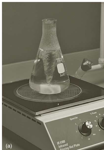
Figure 17.2 Gently heat the sample to remove \text{CO}_2 gas.
