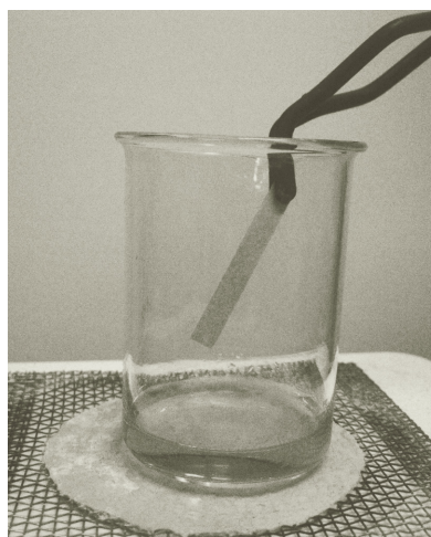
Figure 38.4 Absorbing \text{NH}_3 vapors on red litmus
