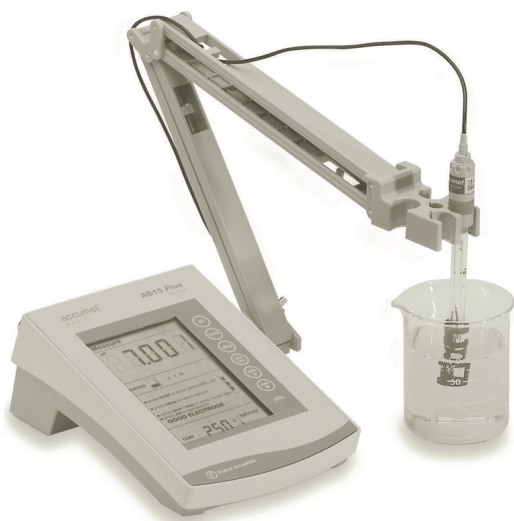
A modern pH meter with a combination electrode
