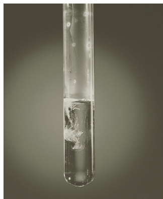
Figure 22.1 The addition of conc HCl to a saturated NaCl solution results in the formation of solid NaCl.
