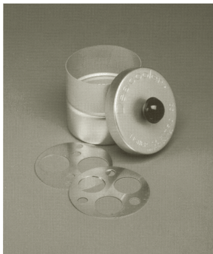
Figure T.15b A simple laboratory desiccator (left) or a glass desiccator (right) contains a desiccant (usually anhydrous \text{CaCl}_2 ) to provide a dry atmosphere.
