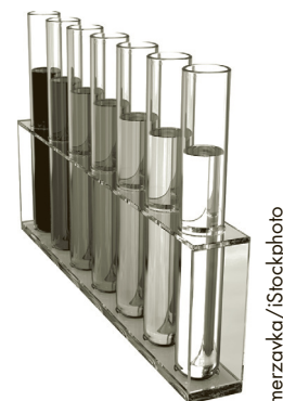
Figure 23.1 The higher concentration of light-absorbing species, the more intense is the color of the solution.
