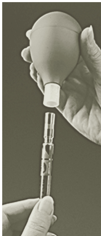
Figure T.16c Draw the liquid into the pipet with the aid of a rubber pipet bulb (not the mouth!).
