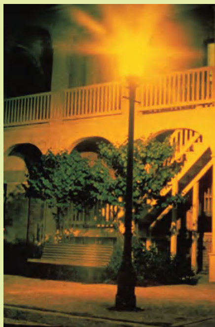
Sodium vapor street lamps are still common in many cities and are easily identifiable by their yellow glow. ( Richard Treptow/Photo Researchers, Inc. )
