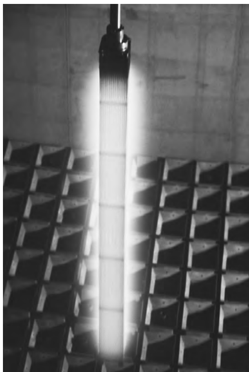
SAMARIUM IS USED IN NUCLEAR POWER PLANT CONTROL RODS, SUCH AS THE ONE SHOWN HERE. (Tim Wright/Corbis. Reproduced by permission.)
