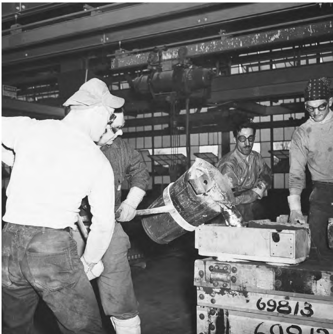
DURING WORLD WAR II, MAGNESIUM WAS HEAVILY USED IN AIRCRAFT COMPONENTS. IN THIS 1941 PHOTO, WORKERS POUR MOLTEN MAGNESIUM INTO A CAST AT THE WRIGHT AERONAUTICAL CORPORATION. (Bettmann/Corbis. Reproduced by permission.)
