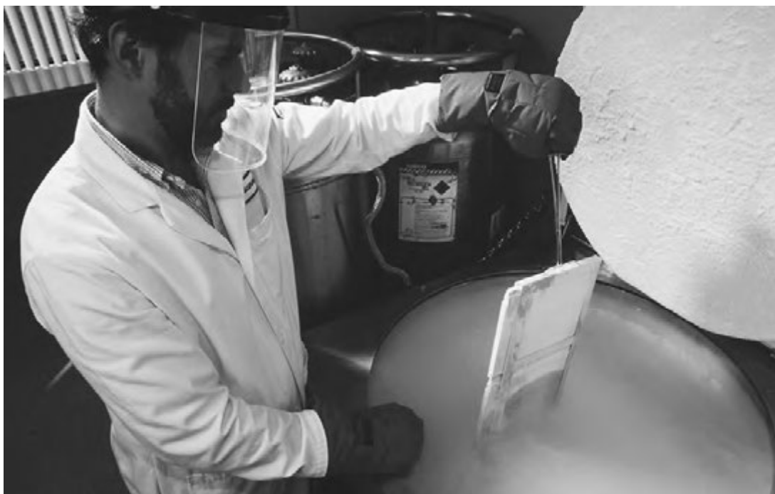
LIQUID NITROGEN ACCOUNTS FOR ABOUT ONE-THIRD OF ALL COMMERCIAL USES OF NITROGEN. HERE, A MEDICAL WORKER PUTS A SAMPLE OF BONE MARROW INTO A TANK OF LIQUID NITROGEN FOR PRESERVATION. (Leif Skoogfors/Corbis. Reproduced by permission.)
