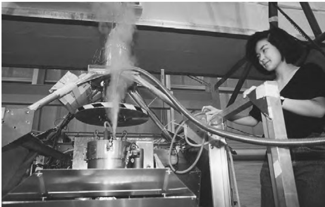
A RESEARCHER WORKS WITH LIQUID HELIUM AS PART OF AN EXPERIMENT ON COSMIC BACKGROUND RADIATION. CLOSE TO ABSOLUTE ZERO, HELIUM TRANSFORMS INTO A HIGHLY UNUSUAL LIQUID THAT HAS NO MEASURABLE RESISTANCE TO FLOW. (Roger Ressmeyer/Corbis. Reproduced by permission.)
