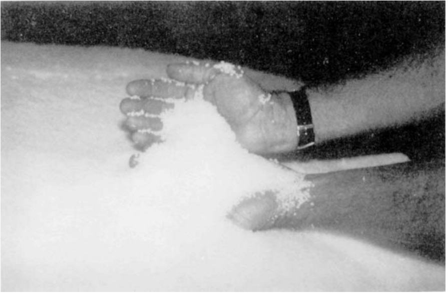
Figure 16.16 Polymers are often pelletized during the extrusion process, a convenient state in which to store and ship plastics before final fabrication. (Courtesy of BP Chemicals, Alvin, Texas)
