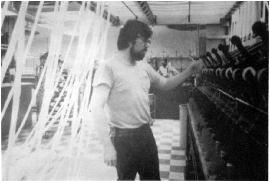
Figure 17.3 Spinning of fibers for use in carpets. (Courtesy of Du Pont)
