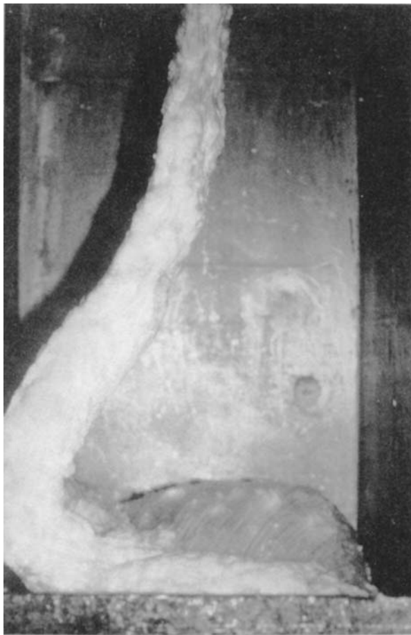
Figure 16.12 Polymer ribbon in a molten state at high temperatures ready to enter an extruder. (Courtesy of BP Chemicals, Alvin, Texas)
