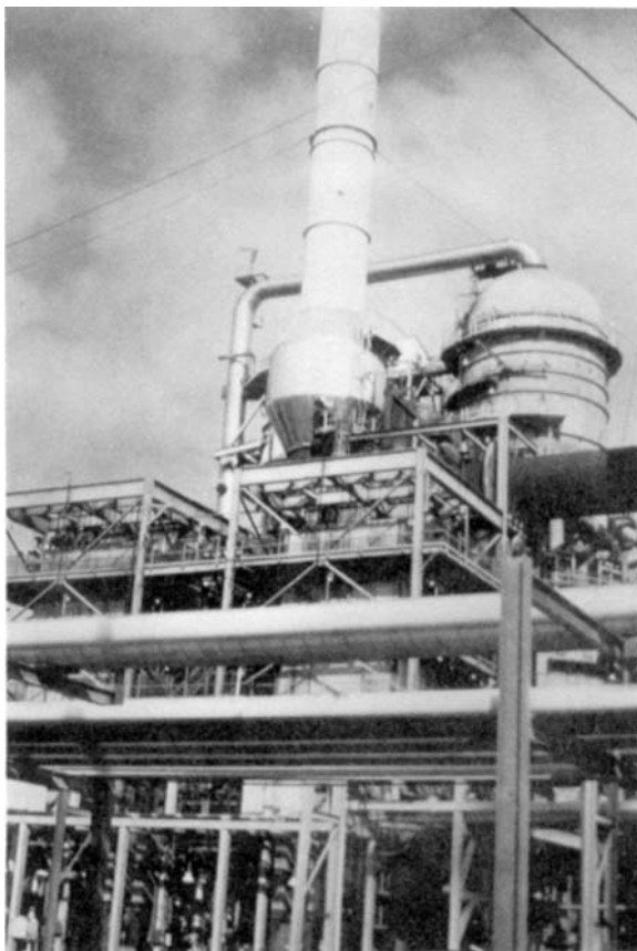
Figure 7.7 A typical large catalytic cracking unit (on the right in this picture) can process 110,000 barrels/day. (Courtesy of BP Amoco, Texas City, TX)
