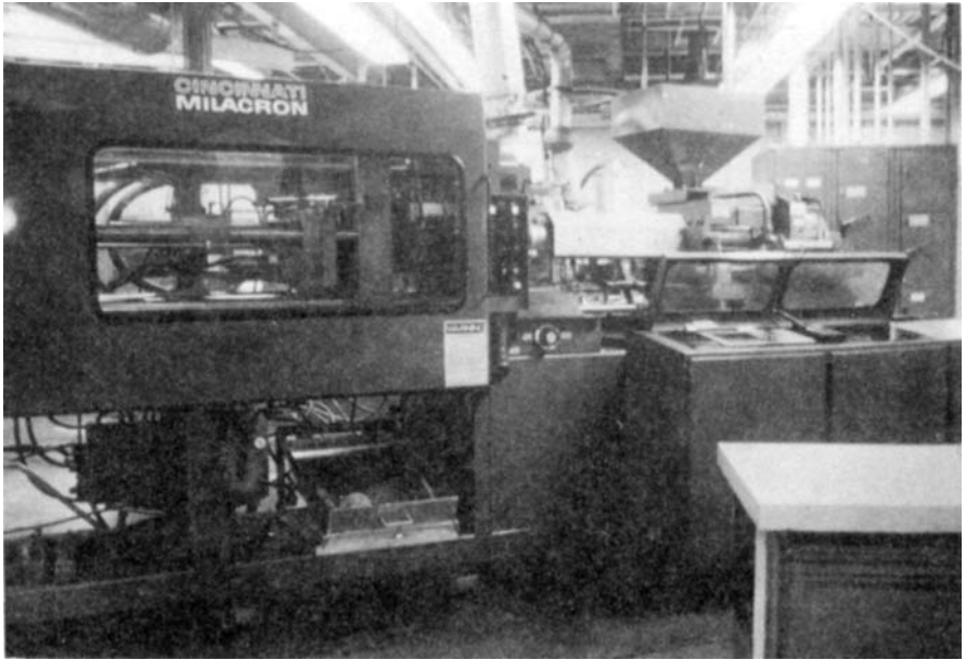
Figure 16.11 Research injection molding equipment. (Courtesy of Du Pont)
